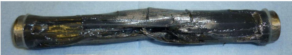
Figure 34 - Specimen 3 after failure. Critical pressure = 105MPa.
