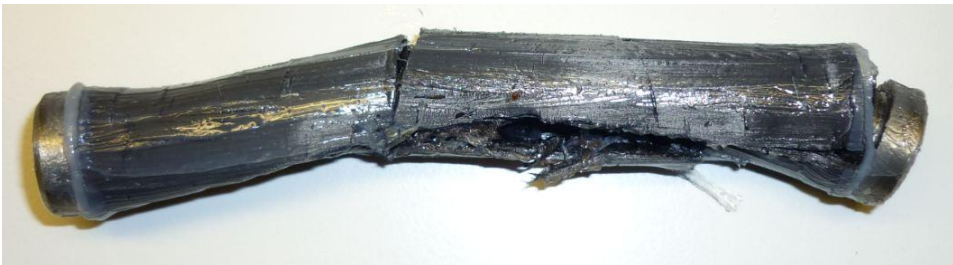
Figure 35 - Specimen 4 after failure. Critical pressure = 70MPa.
