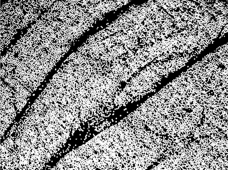
Figure 48 – Rendered image of hoop fiber layer in specimen nr2, with 100x enhancement. Estimated volume fraction: 0,558.
