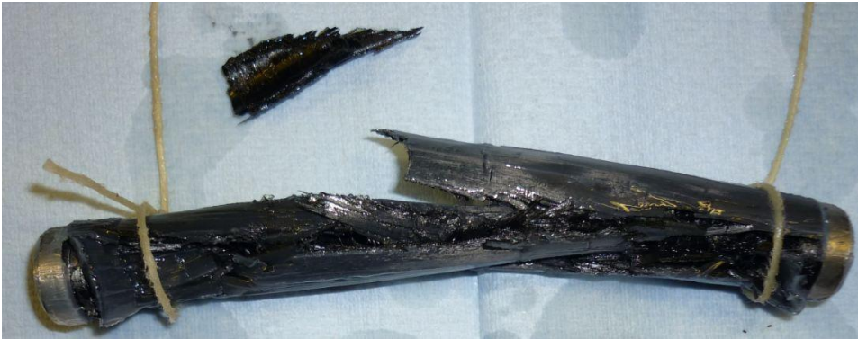
Figure 36 - Specimen 6 after failure. Critical pressure = 53MPa.
