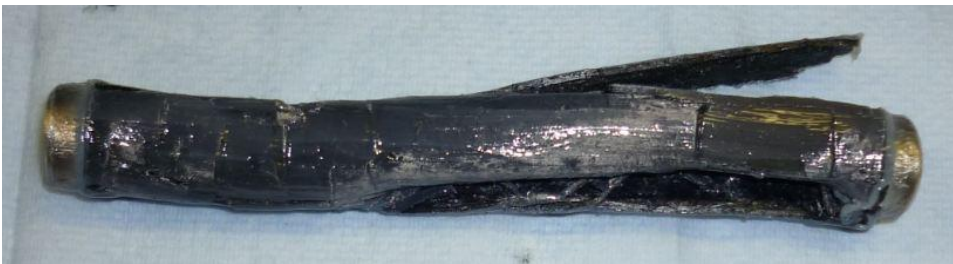
Figure 33 - Specimen 2 after failure. Critical pressure = 91MPa.
