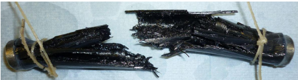
Figure 37 - Specimen 8 after failure. Critical pressure = 69MPa.
