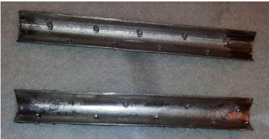
Figure 24 – The moulds used for specimen production using approach 2. The holes in the mold facilitate escaping of superfluous resin.
