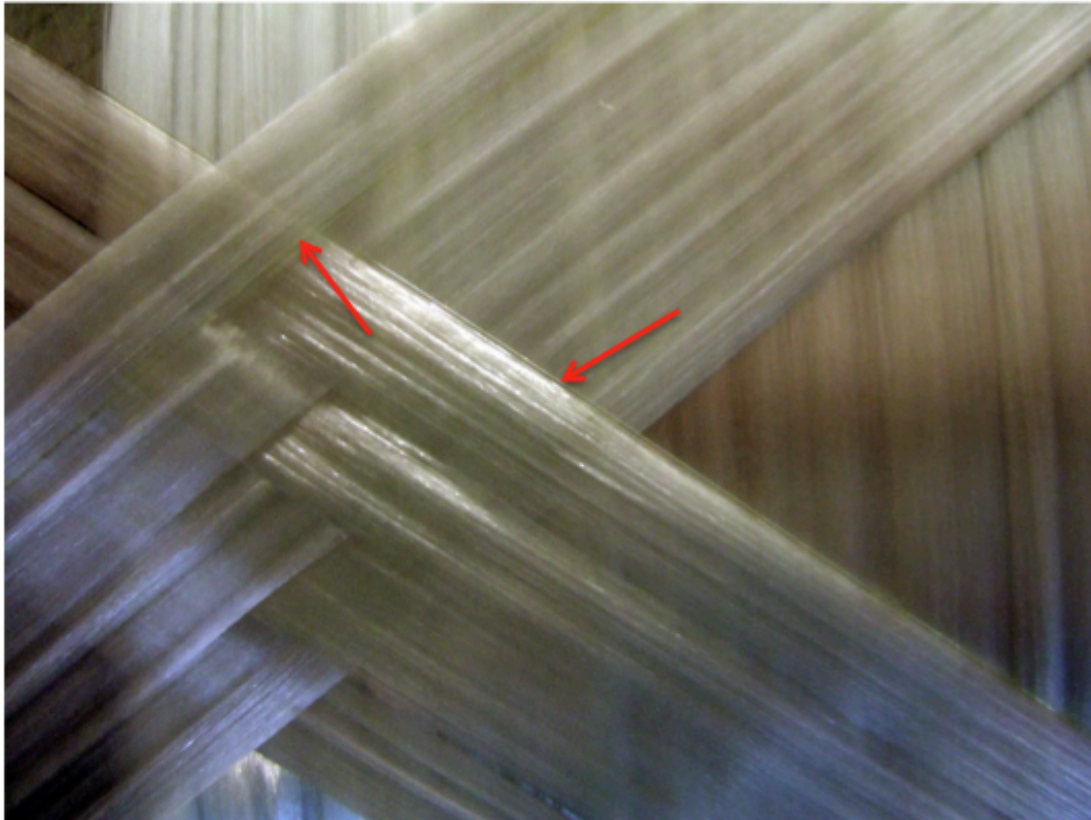
Figure 38: Close up of filament winding with fibre optical cable barely visible at the tip of the arrows.
