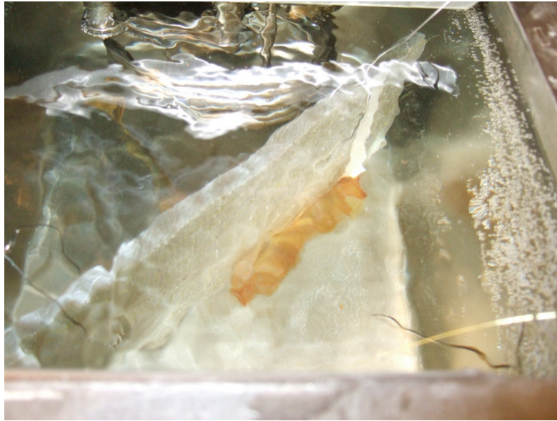
Figure 30: Temperature measurements in a temperature bath using fibre optical sensor.
