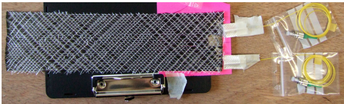
Figure 58: Patch of crack 2 with fibre sensors.
