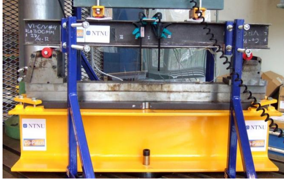
Figure 3. Experimental setup at NTNU Fatigue lab of the patched IPE100 beam.
