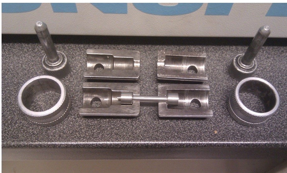
Figure 48: The attachments used for mounting the small specimens.
