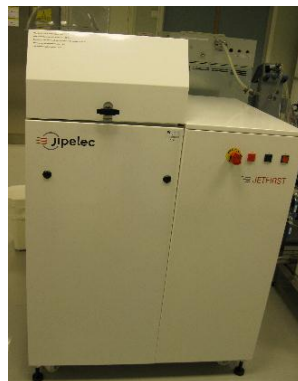
Figure 5.5: The JetFirst 200 RTP unit [108]
