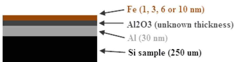
Figure 6.9: Illustration of deposited layers for most samples. Some have been grown without the Al and Al 2 O 3 layer
