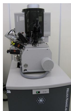
Figure 5.9: The FEI Helios DualBeam Focused Ion Beam microscopy – FIB [113]
