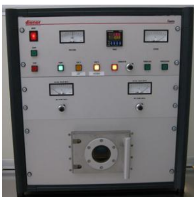
Figure 5.7: The Femto plasma cleaner (Diener Electronics) [110]
