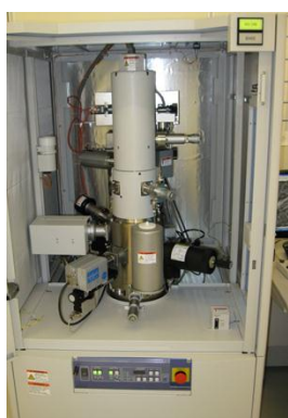
Figure 5.8: The Hitachi S-5500 Scanning Transmission Electron Microscopy – S(T)EM [112]
