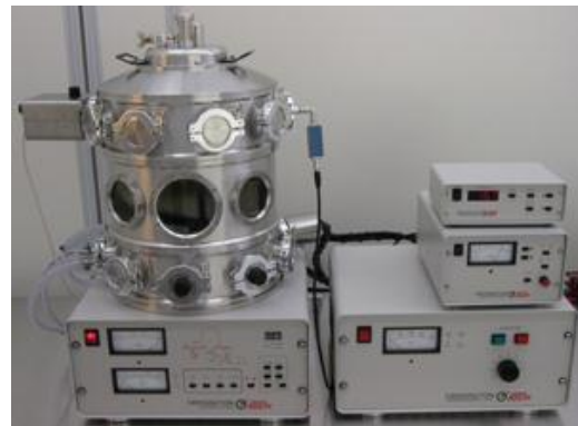
Figure 5.4: Cressington 308R Sputter and Evaporator [107]
