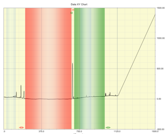
Figure 6.8: Measurements with the profilometer on a 30 nm thick Fe film, where the green bar is placed on the right side of the valley
