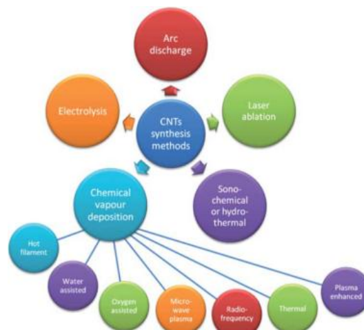
Figure 2.1: Overview of the synthesis methods for CNTs [30]. A figure of higher quality can be seen in Appendix A
