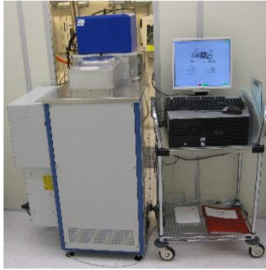
Figure 5.6: The PlasmaLab System 100 PECVD (Oxford Instruments) [109]
