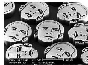
Figure 2.13: Face of President Obama synthesized by growing vertically aligned CNTs on a patterned catalyst. Each face consists of about 150 million parallel CNTs. By patterning the catalyst, CNT can be grown out of selected regions on the substrate [32]
