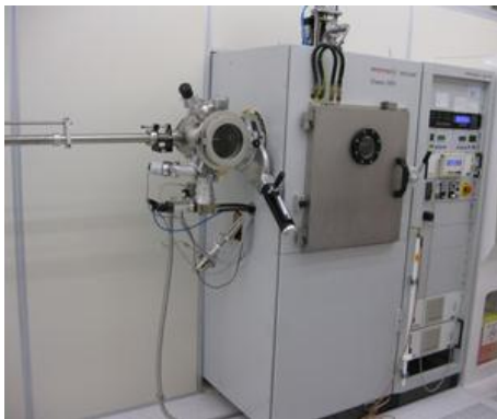
Figure 5.3: The Pfeiffer Vacuum Classic 500 e-beam evaporator [106]
