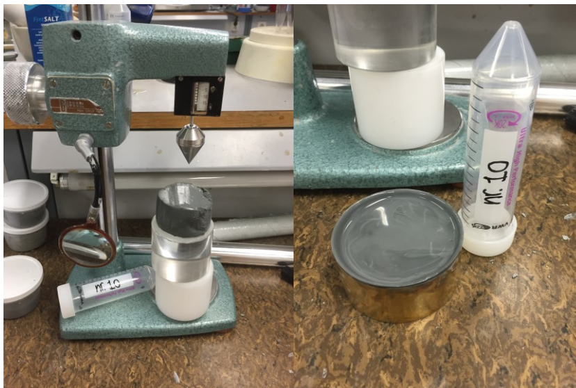
Figure 6-13 Cone test for sample 10 with 60g/60° cone for C_u and 10g/60° for C_{ur} , respectively.
