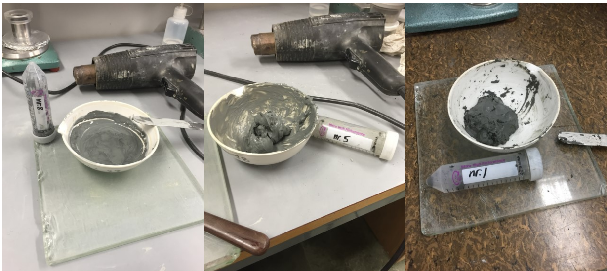
Figure 6-27 The difference of the remolded clay after stirring the saltwater back into the clay for sample 8, 5 and 1, respectively.
