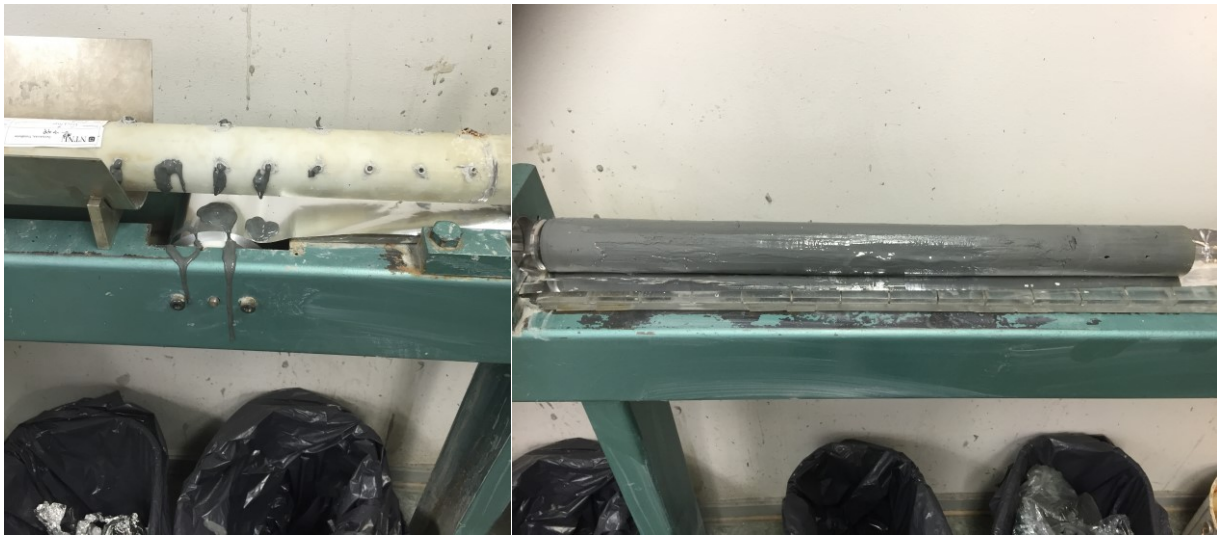
Figure 6-11 The clay moving out of the perforated holes in cylinder A and the end result, respectively.
