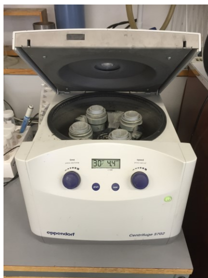
Figure 6-17 Centrifuge 5702 from Eppendorf, with speed 4,4 rps
