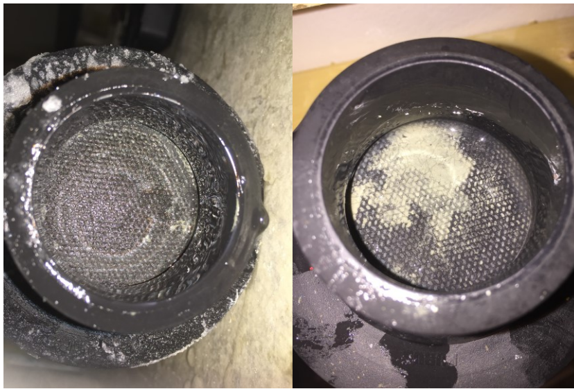
Figure 6-8 The filter of the lower and upper part of the clay in cylinder A after testing, respectively.
