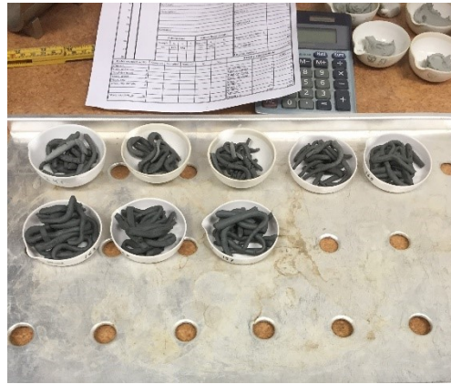
Figure 6-28 Finding the plasticity index of the clay
