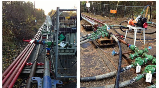
Figure 3. Flow-loop setup components for drillstring washout and gas injection (left) and for drill bit nozzles (right).
