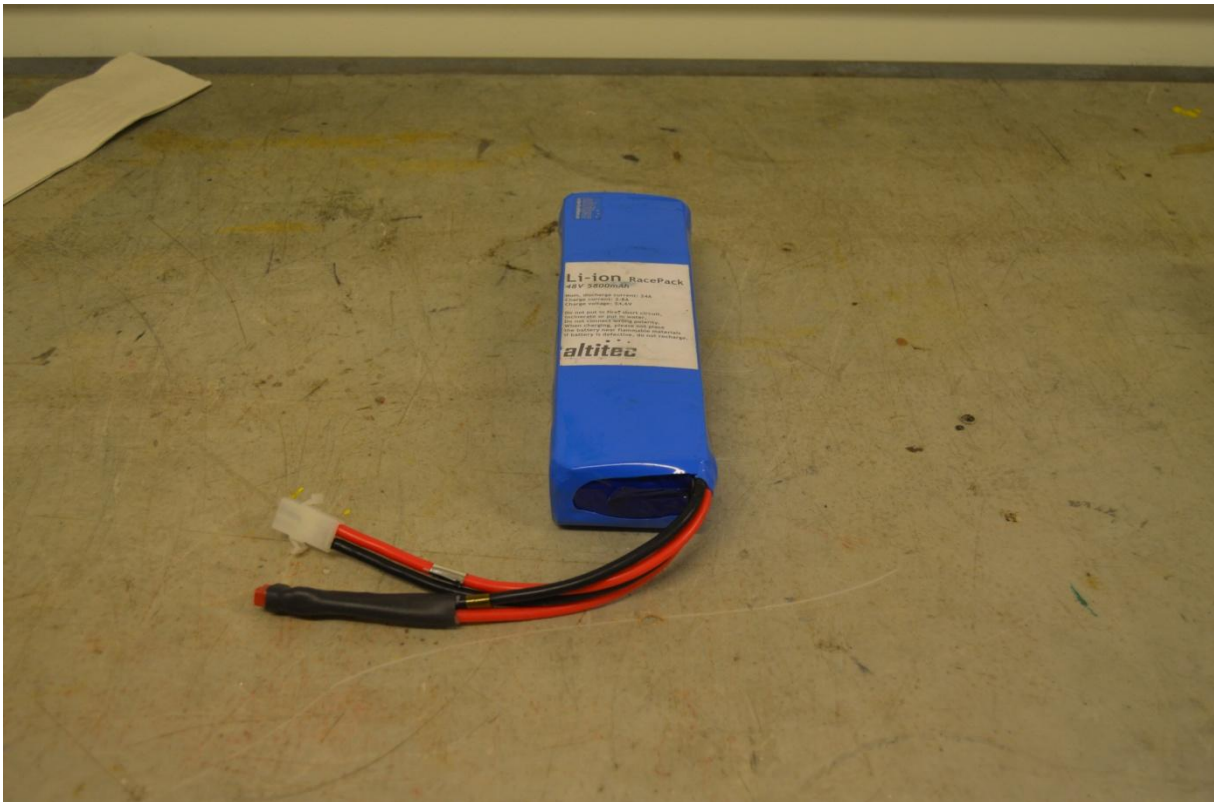
Figure 24 Altitec's battery pack
