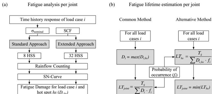
Fig. 3. (a) Standard and extended approach to predict fatigue damage ( $D$ ) in tubular joints, (b) common and alternative method to estimate fatigue lifetime ( $LT$ ) as defined in this paper. Index  $i$  describes a load case with a simulated length of  $T_s$ .
