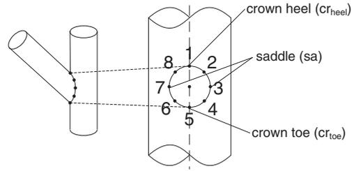
Fig. 2. Positions of hot spots in tubular joints
