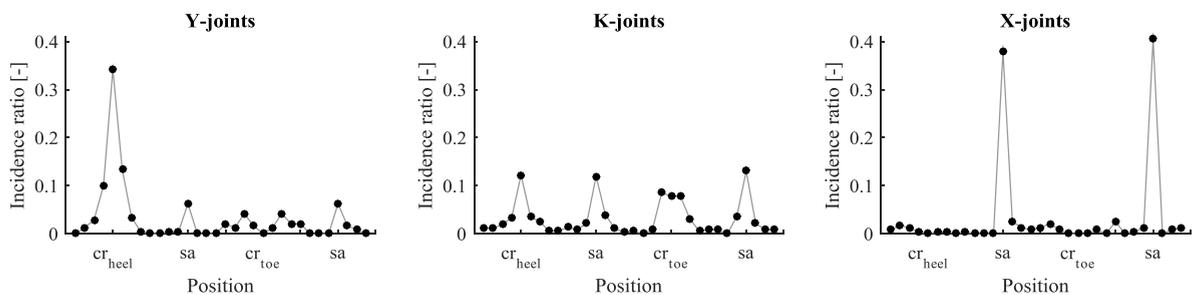
Fig. 5. Incidence ratio of highest fatigue damage per joint type plotted against the position around the circumference of the joint. Position of the crown heel ( $cr_{heel}$ ), saddles (sa), and crown toe ( $cr_{toe}$ ) are marked on the horizontal axis.
