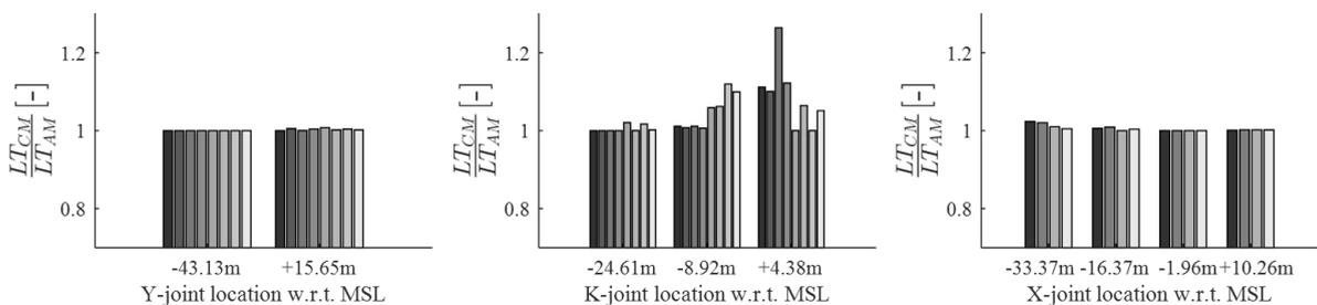
Fig. 6. Ratio for estimated fatigue lifetime (LT) between common method (CM) and alternative method (AM) for different types of joints. The joints are grouped per height with respect to (w.r.t.) mean sea level (MSL).
