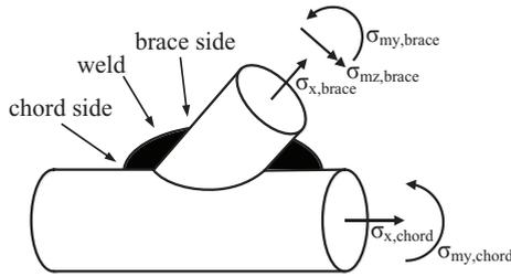
Fig. 1. Stresses and weld at tubular joint
