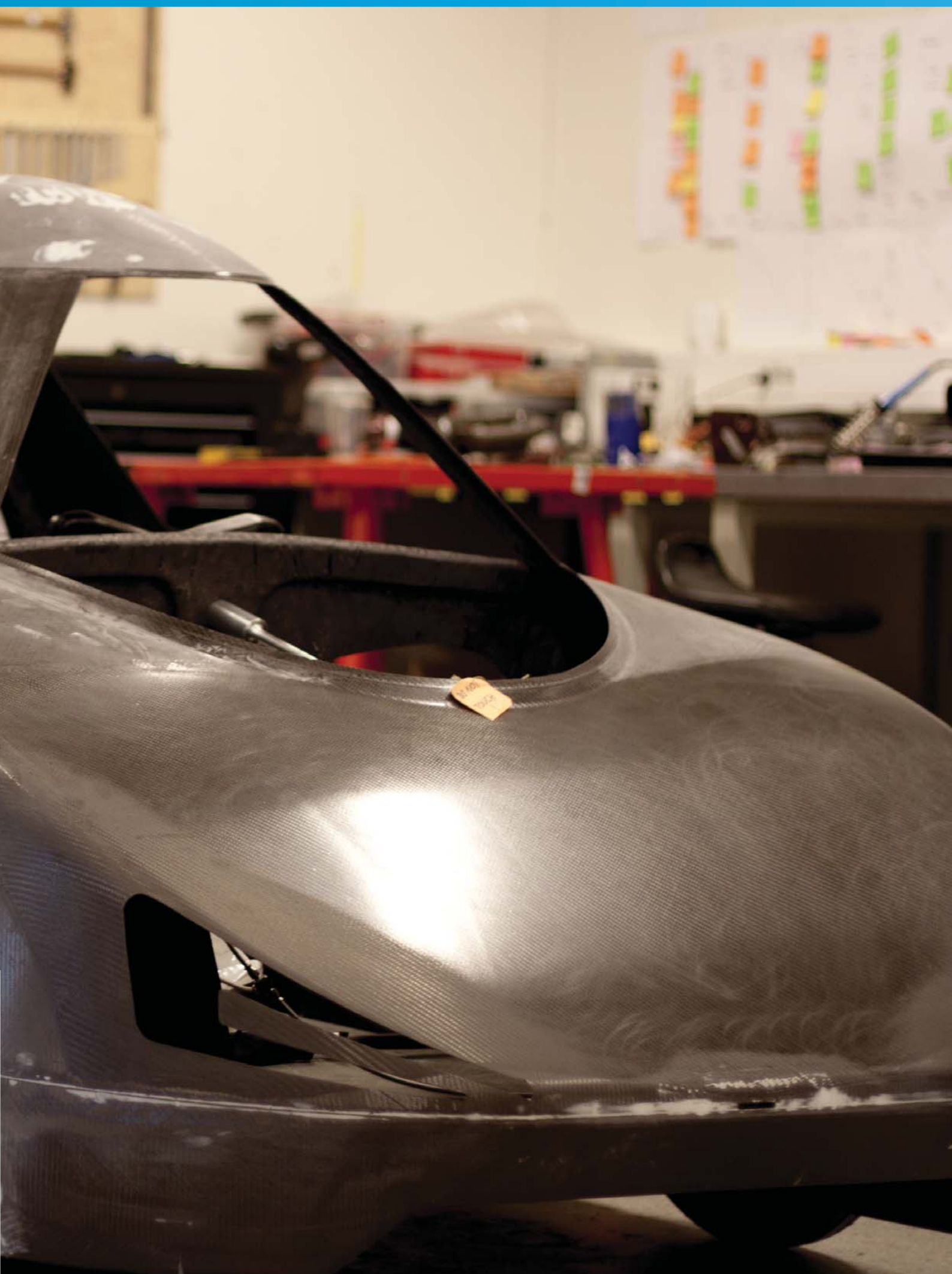
The monocoque was already designed and in production when the design of the interior started
