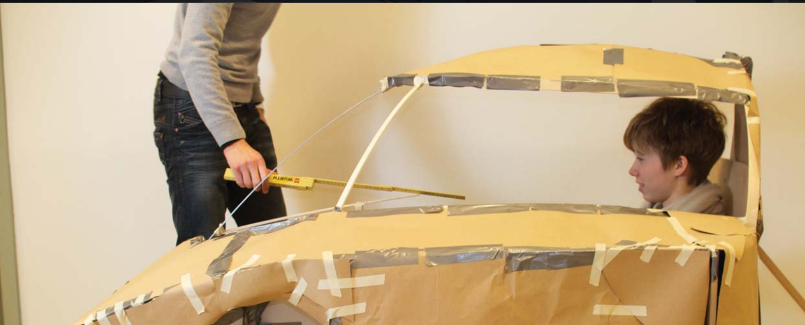
A full scale mock-up was used for testing before the monocoque could be used for this purpose
