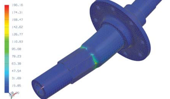
Figure 3.7.6: FEM analysis of motor axle subject to a hard bump
