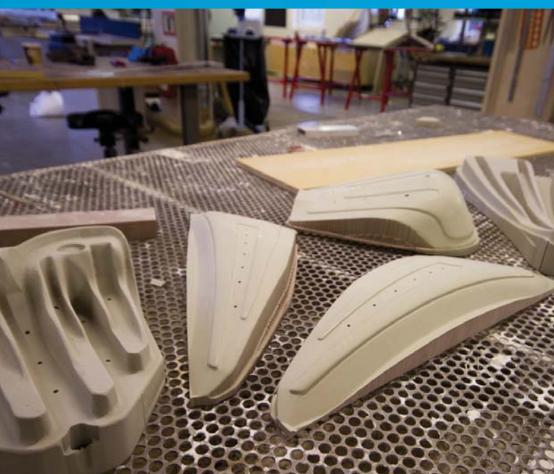
8 different molds were made to vacuum form all the parts for the lights
