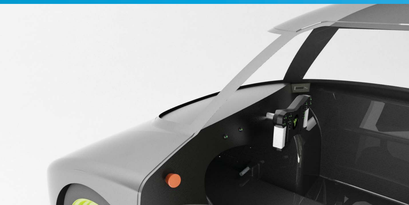
The final design of the dashboard, containing two different parts; the top cover and the front beam.
