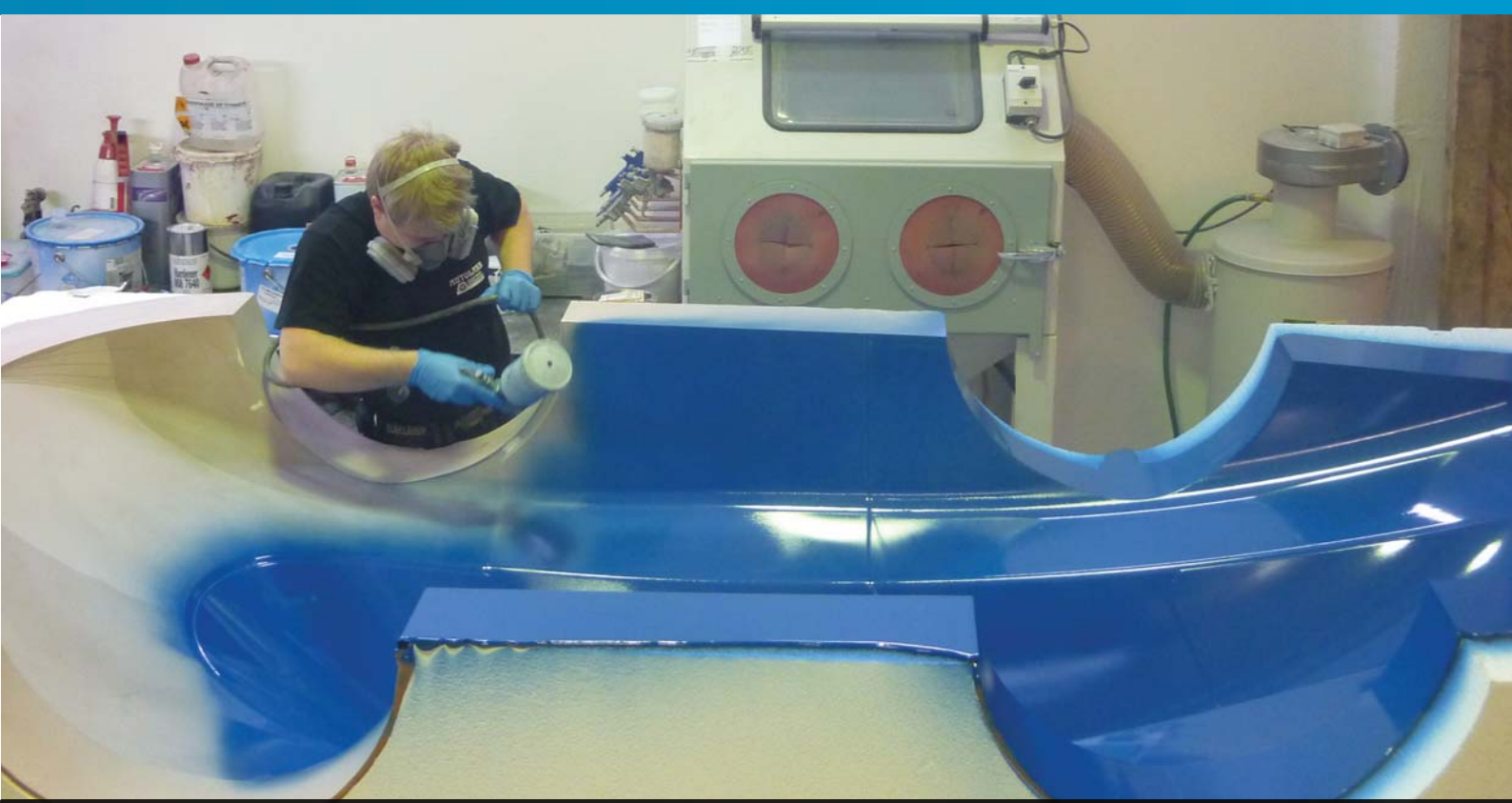
Finished prepared molds, treated with a layer of blue polyurethane paint at HPC
