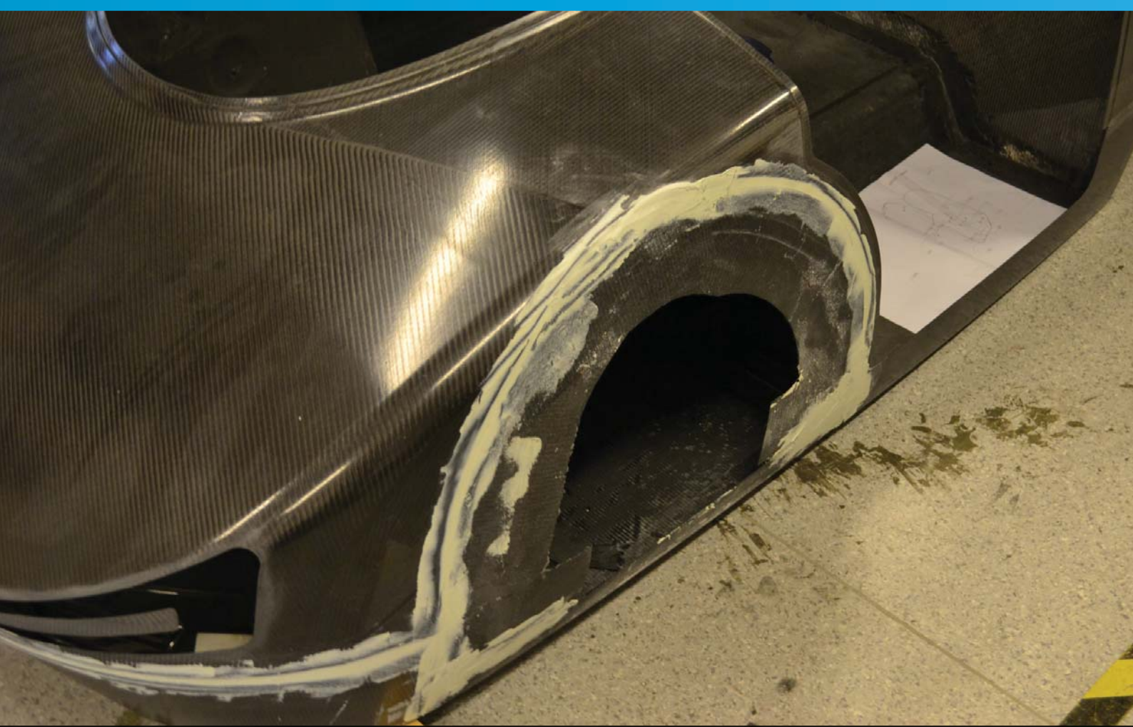
Body filler applied around the front wheel well cover
