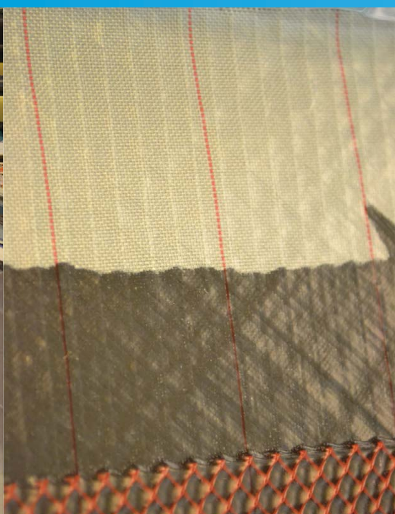
Resin flow mesh at the edges of the mold, the resin slows down considerable
