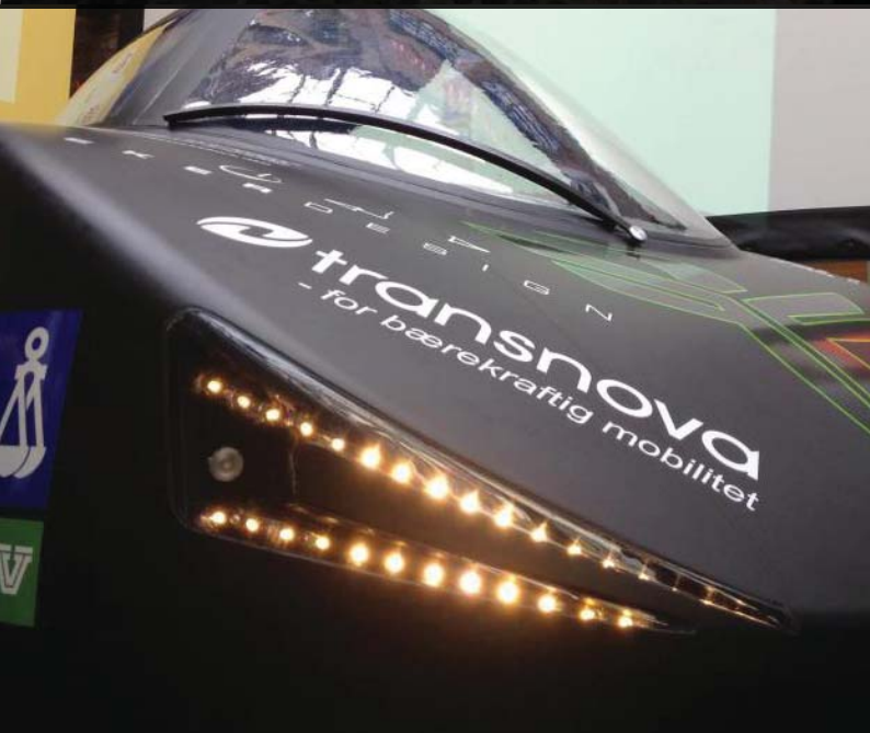
The final front and rear lights mount in the finished car. The lights are attached to the car with velcro on the inside.
