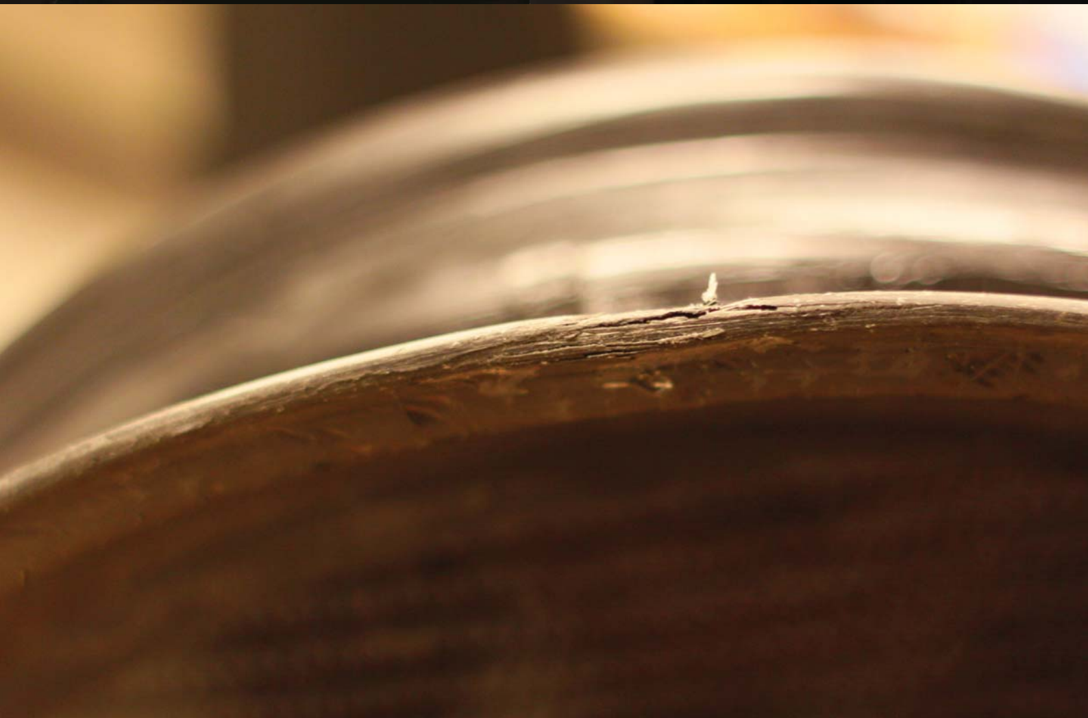
The crack in the broken rim after testing at Dragvoll
