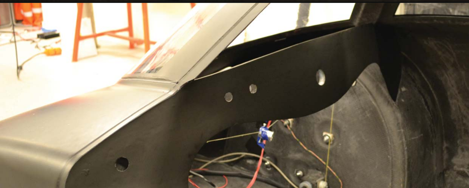
The finished dashboard with holes for emergency shut-off button, start/stop button, windshield wiper button and steering rod.
