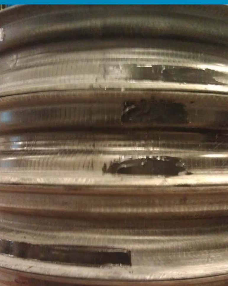
Left: Araldite 2031 to cover up small cracks and irregularities on the rim rings inner surface Right: Sikaflex and PVC tape to prevent leakage
