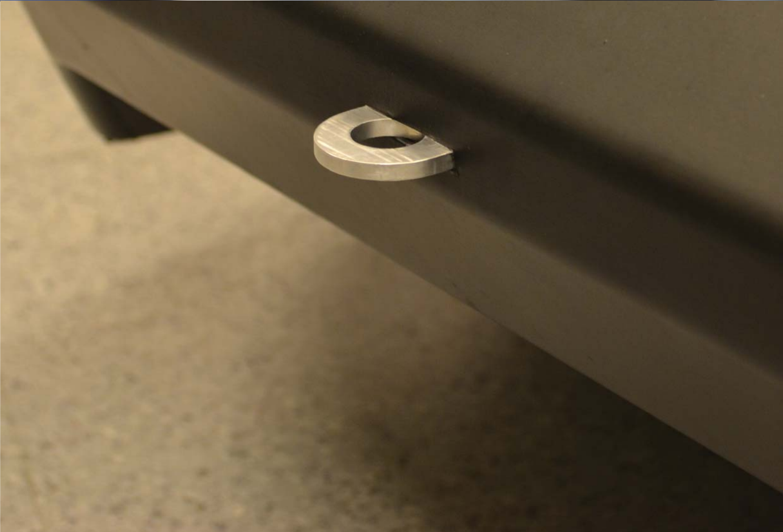
Top: Towing hook of the DNVFF, threaded bar solution. Bottom: Final design of the towing hook installed to the DNVFF2. One aluminum part.
