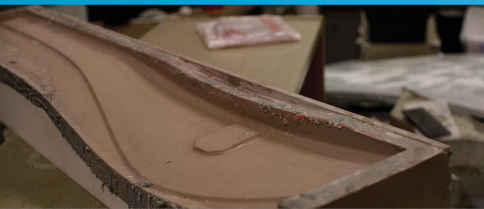
The mold was milled out of Ebaboard with a CNC-milling machine
