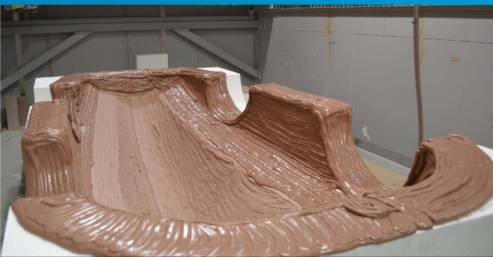
Epoxy paste finished laid at the top part. The difference between P25 and P26 is clearly shown (P25 in light brown)
