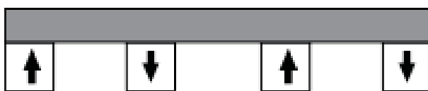
Figure 3.7.12: Magnets in a Hallback array, arrows showing direction of magnetization
