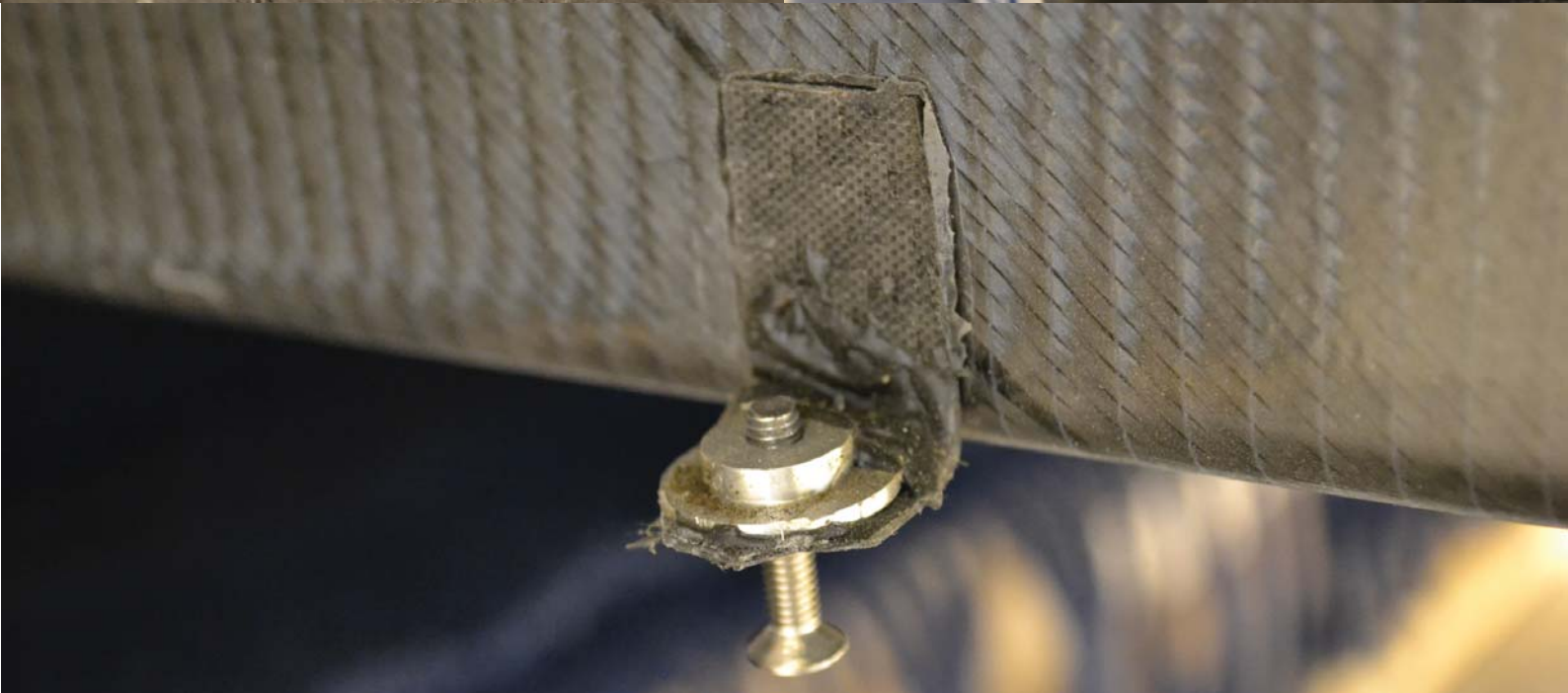
Top: Rubber band connecting the side cover and wheel well. Middle: Aluminum fixings on side cover and wheel well. Carbon fiber stopper used to secure the side cover. Bottom: Screw connections securing the cover in the tunnel, underneath the car.
