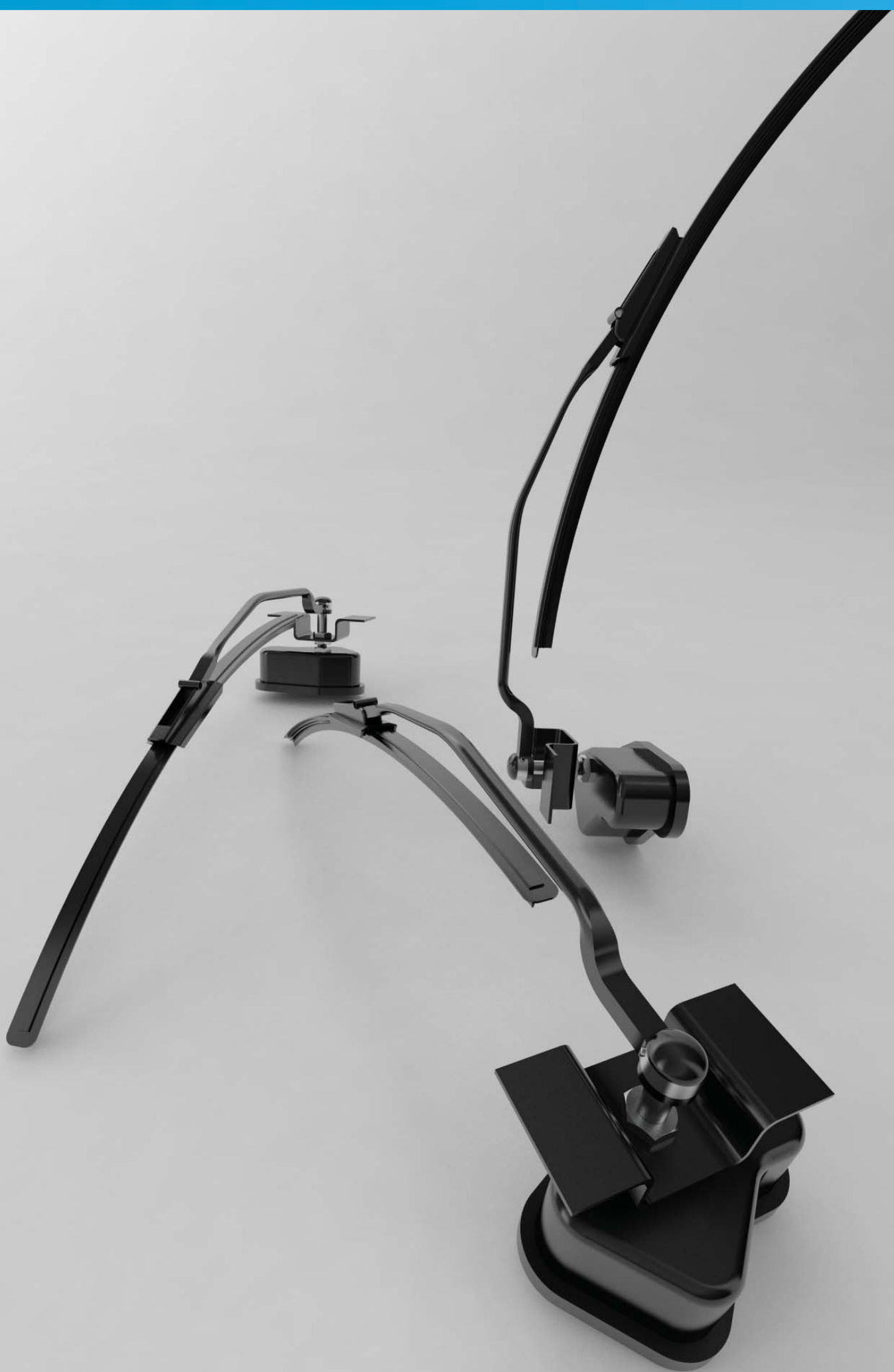
Final windshield wiper design with wiper motor, wiper blade and wiper arm.
