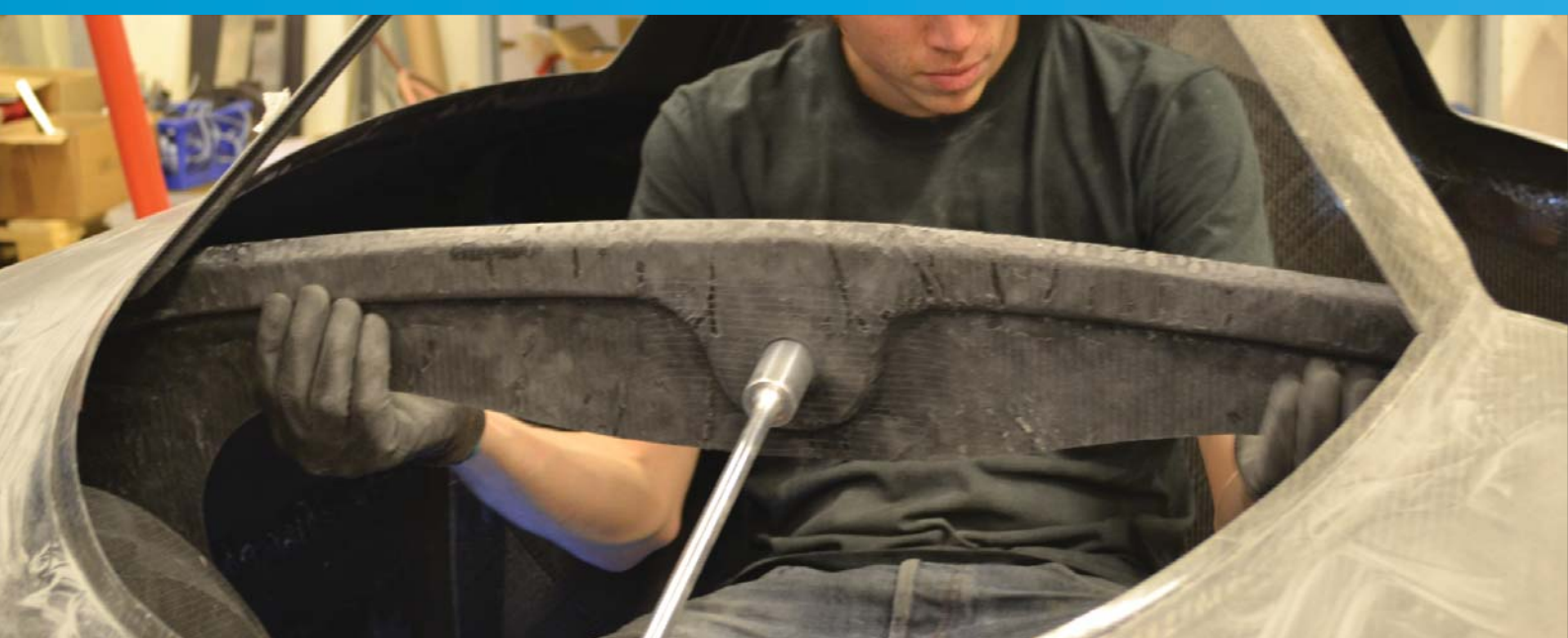
The front beam of the dashboard was glued on to the wheel wells. The reinforcement with a foam core made it stiff enough to support the steering wheel.
