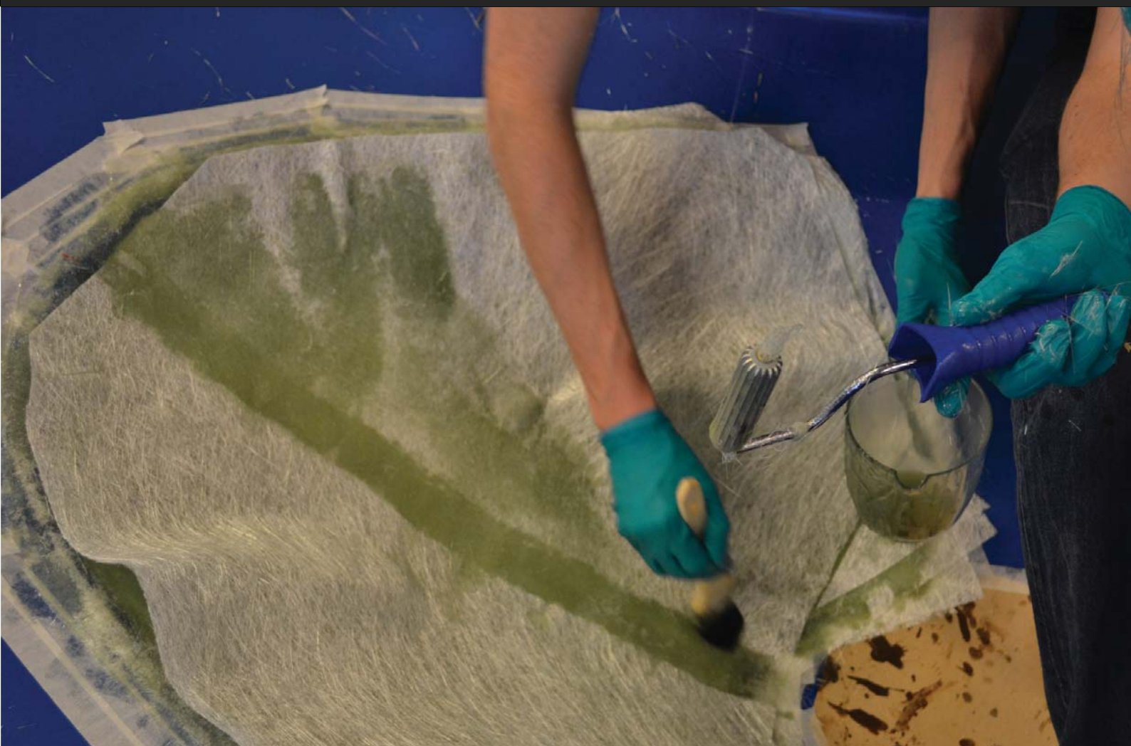
After a quick hardening of the gel-coat, several layers of fibreglas infused with polyester was applied
