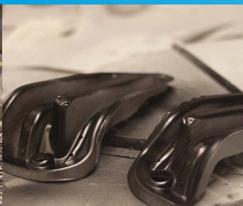
The inside of the lights were vacuum formed in transparent PET, while the outside were made of poly carbonate.
