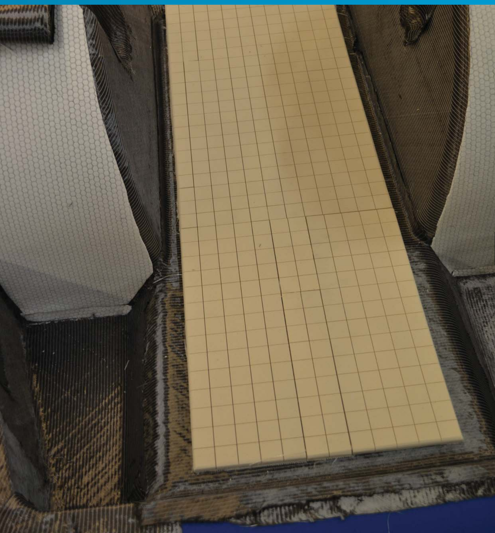
10 mm thick Divinycell core in floor and 3 mm thick Sorix core in the wheel well perimeter
