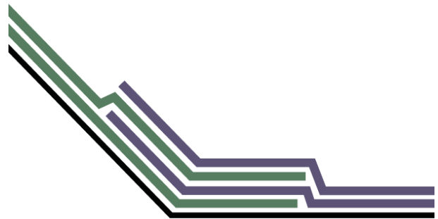
Figure: 3.1.8: Overlay in a corner, two layer layup leads to four layers in the splice area.
