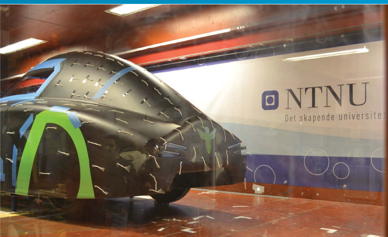
The car during wind tunnel testing. Tufts located over the top remained still, tufts flapping at the sides due to flow separation after the open front wheels.
