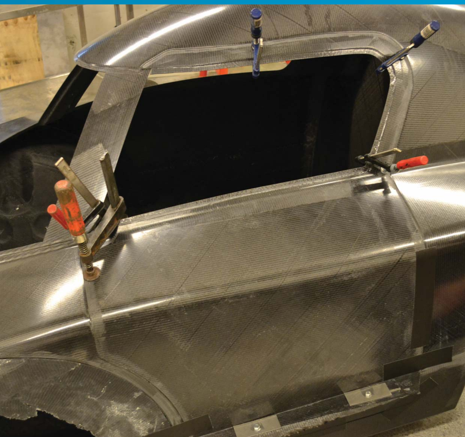
Reinforcing the door with 50 mm wide Rohacell 31 core
