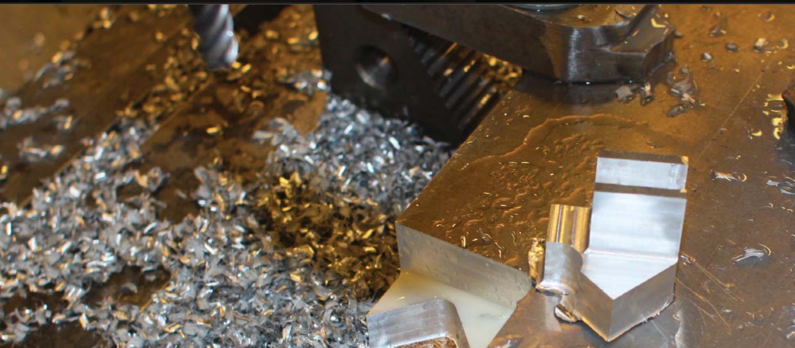
One of the lower A-arm connectors milled out in the Makino CNC milling machine
