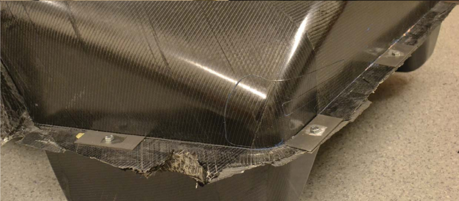
Screw connection plates were made to hold the two parts together
