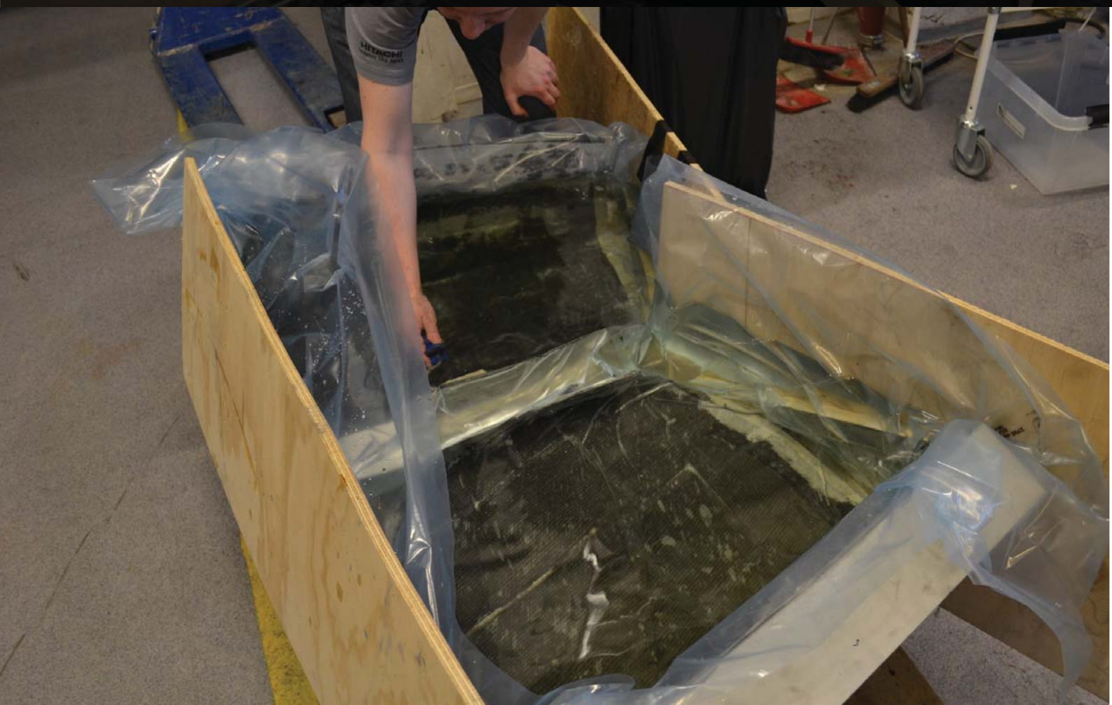
Water reservoir method used to produce rear wheel well covers
