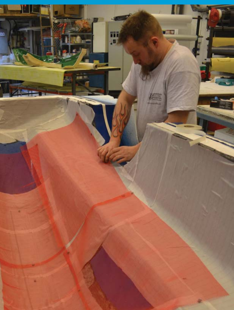
Resin flow mesh, held in place with pieces of vacuum sealer tape
