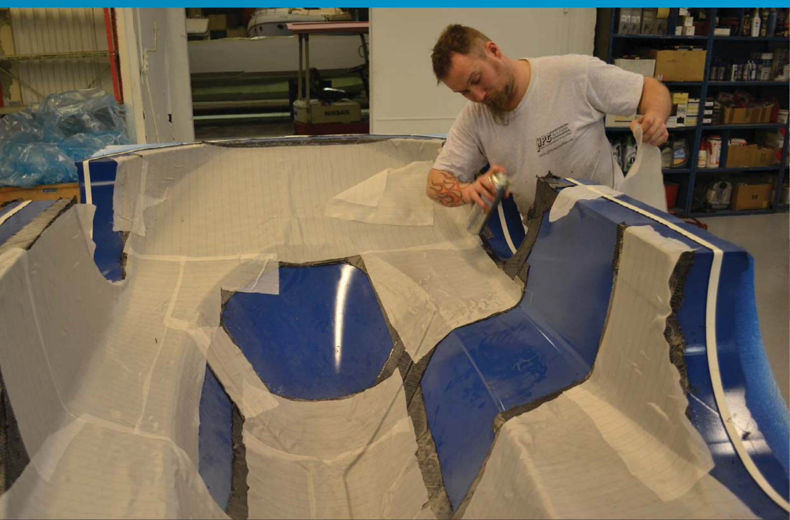
Peel ply applied to the top part, held in place with textile spray glue
