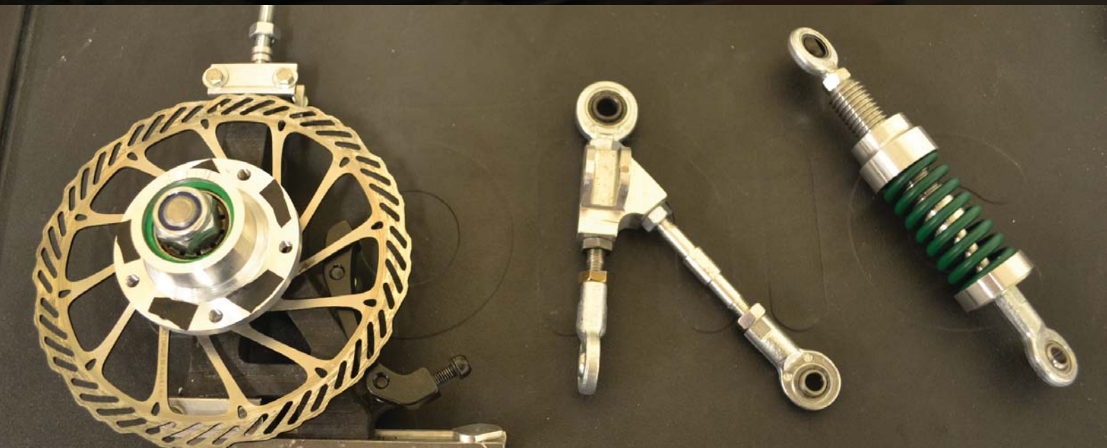
From the left: Knuckle with hub assembly, lower A-arm assembly, coilover assembly
