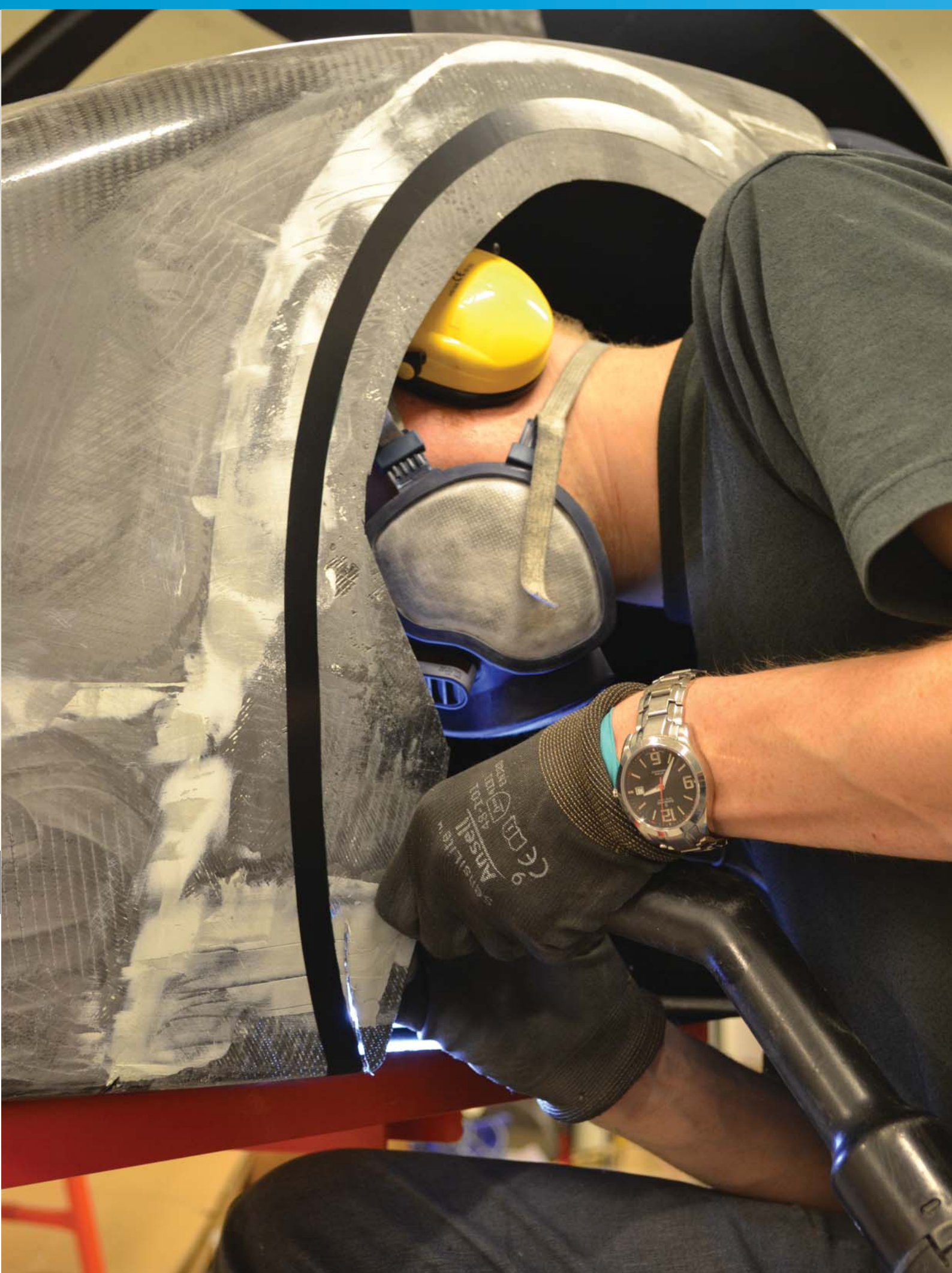
Fine cutting of the wheel well covers, Dremel cutting tool and vacuum cleaner is used
