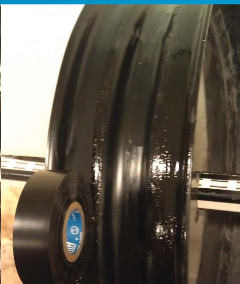
Left: Araldite 2031 to cover up small cracks and irregularities on the rim rings inner surface Right: Sikaflex and PVC tape to prevent leakage
