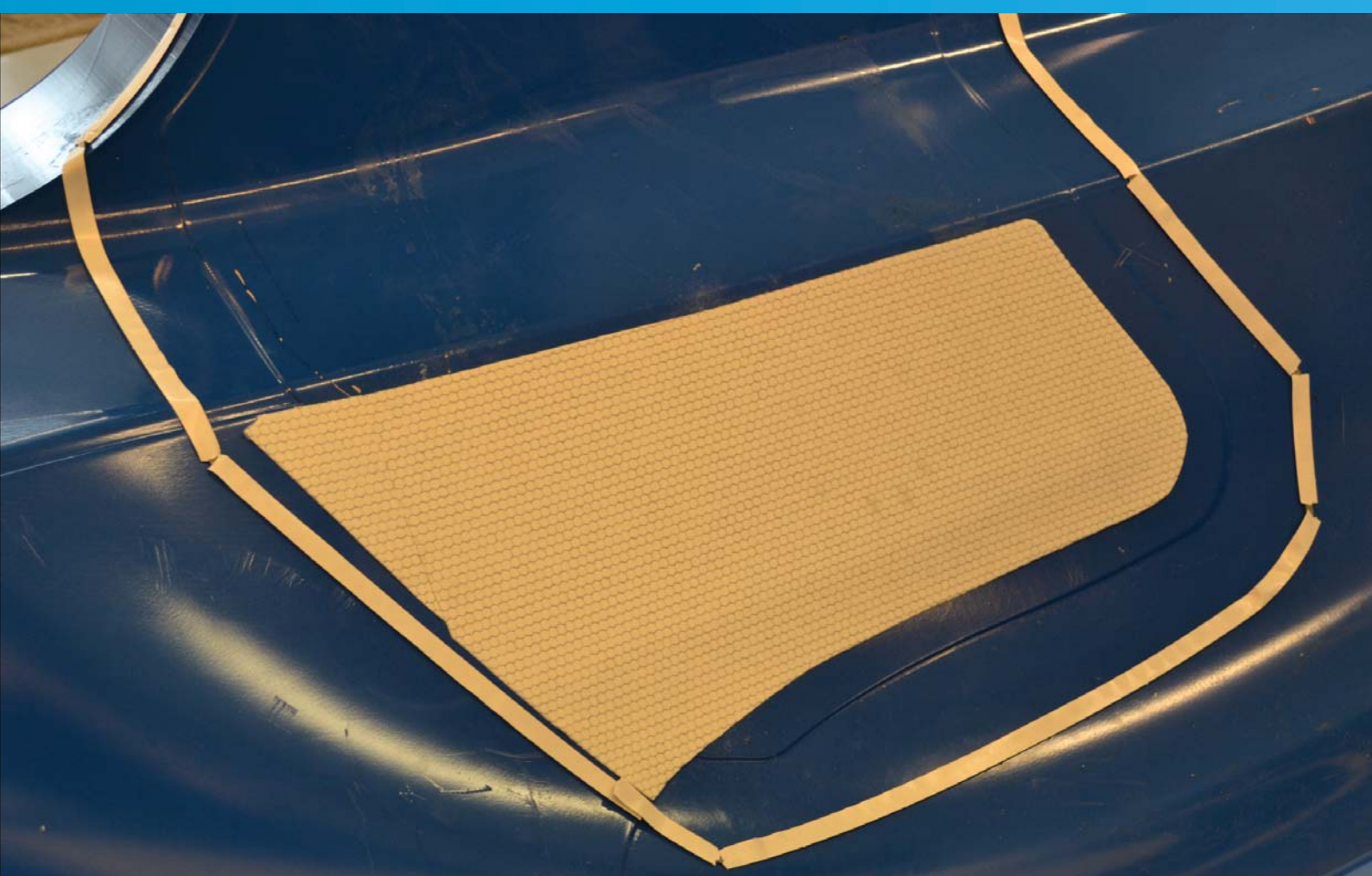
Indent made for the window with the use of 3 mm Sorix
