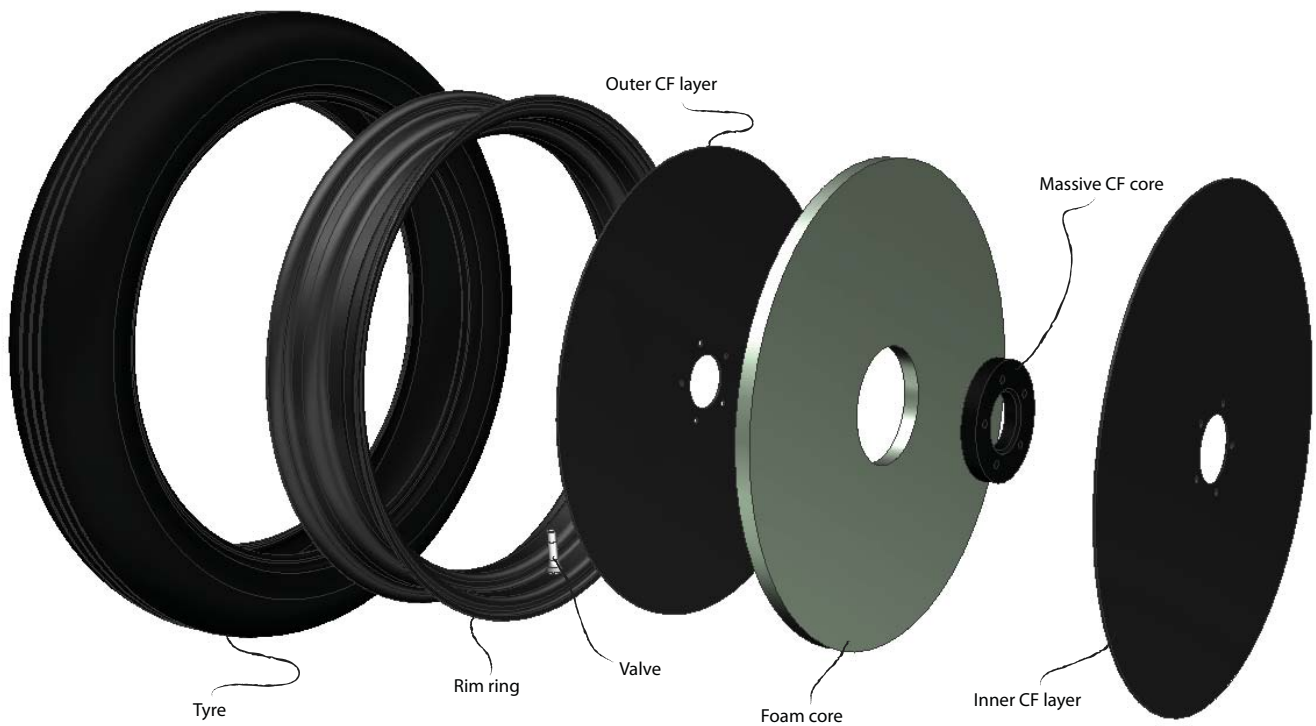
Figure 3.6.1: Exploded 3D CAD model of the rims produced in 2012
