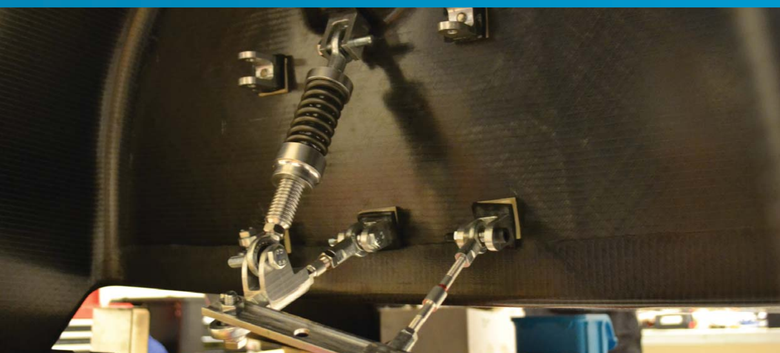
Clevises, lower A-arm, toe link, to link extensor and coilover mounted in the right wheel well
