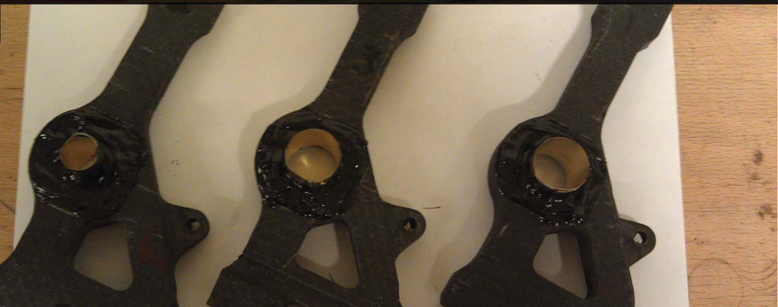
Glue applied on the knuckles uneven surfaces metal sheet formed to a tube to prevent glue from entering the axle hole
