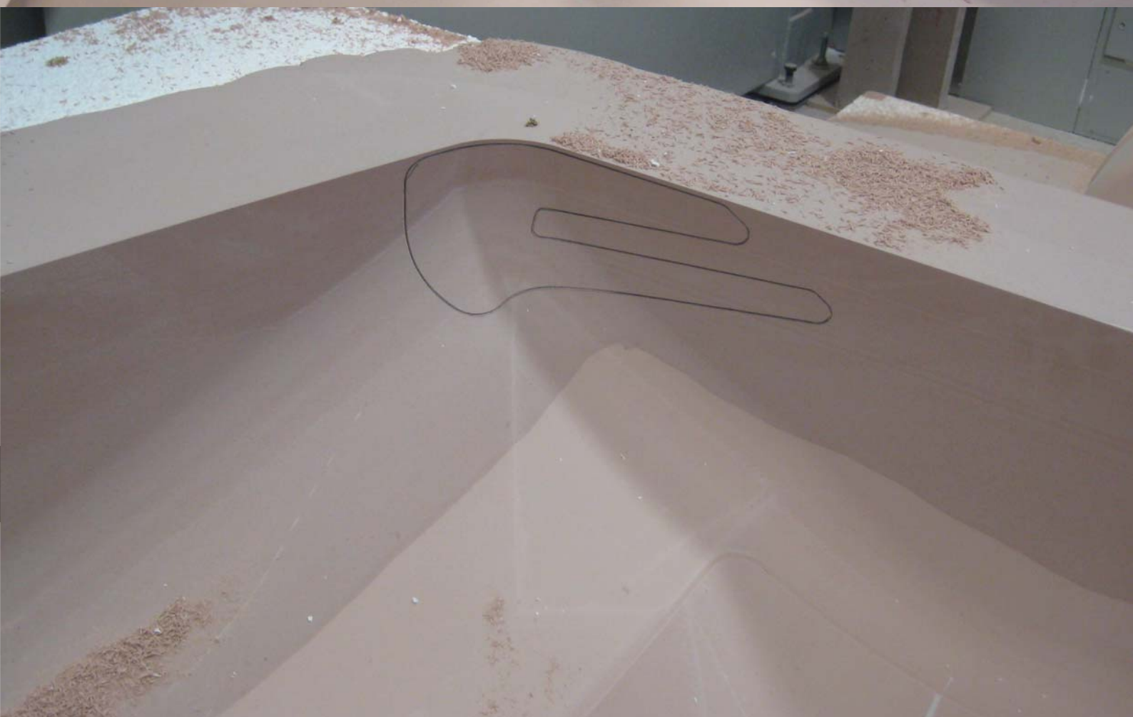
Tracing of lines for the lights was the final step for the milling machine
