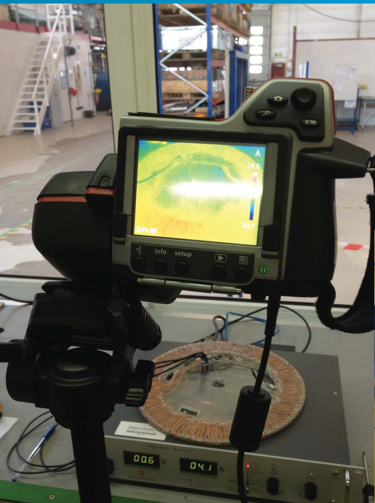
Thermal camera used to examine the first stator when it was exposed to high current
