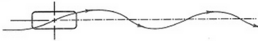
FIGURE 8 – WHEEL TRACKING DUE TO SCRUB RADIUS
