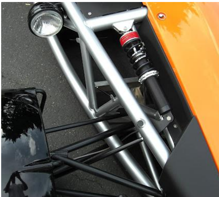
FIGURE 20 – ARIEL ATOM FRONT SUSPENSION DETAIL
