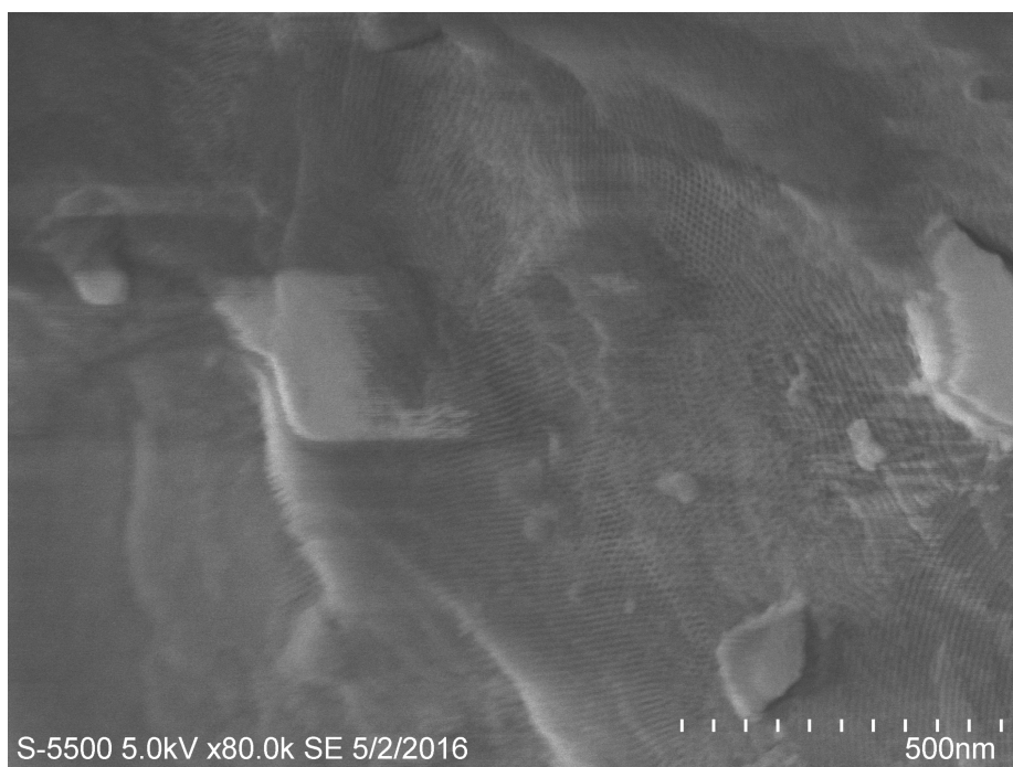
Figure 4.29: SE image of surface and pore structure of m\text{-Al}_2\text{O}_3\text{-1} . A closer view of the pores are presented in Figure 4.30.
