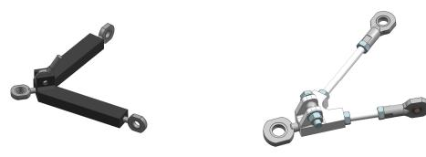
Figure 38: Solid lower wishbone
