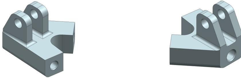
**Figure 40: 3D views of the left wishbone connector**
