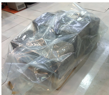
Figur 4.3: Prøvestykker under herding.
