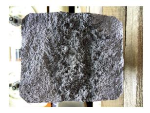
Figure 9: Cross section of a broken  $120\,\mathrm{mm}\,\times\,140\,\mathrm{mm}$  specimen.
