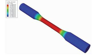
Fig. 2. Stress distribution in Ø16 fatigue specimen.
