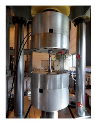
Figure 7: Experimental set-up for fatigue testing of  $\varnothing 21$  specimens.
