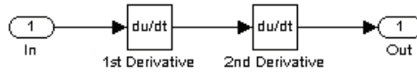
Figure 8: System of double derivation modeled in Simulink using the Continuous Derivative block.
