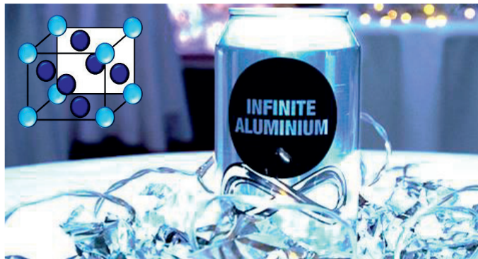
Figure 2.1 Crystal structure of a unit cell in fcc aluminium next to a beverage can made out of aluminium. The light blue atoms are situated at the corners of the unit cell, while the dark blue atoms are situated at the faces.
