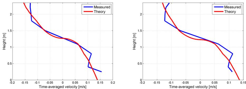
Figure 3: Time-averaged velocity profile for the convector without fan (left) and the panel heater (right) placed at position n°1.
