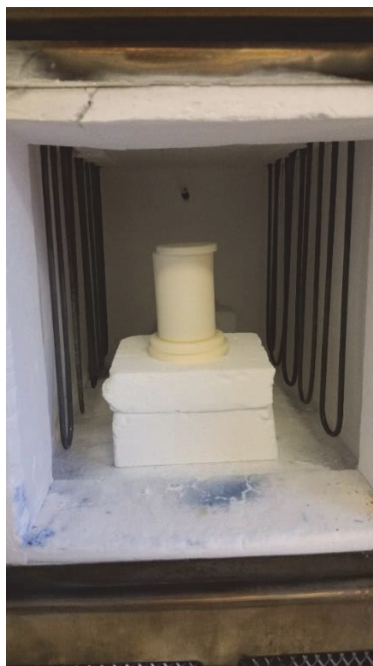
Figure 15: Setup in the high temperature furnace.
