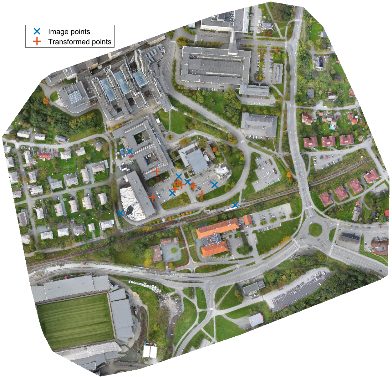
Figure B.13: Lerkendal - Umeyama - without rematching: Shows the orthophoto “Lerkendal” . The blue crosses indicate the areas considered to be a GCP by the prototype when the algorithm proposed by Umeyama (1991) was used to find the absolute orientation. The orange pluses were calculated from the inverse absolute orientation parameters obtained from Umeyama. The measured-in coordinates of the CM where then inverted to image coordinates and displayed as orange pluses.
