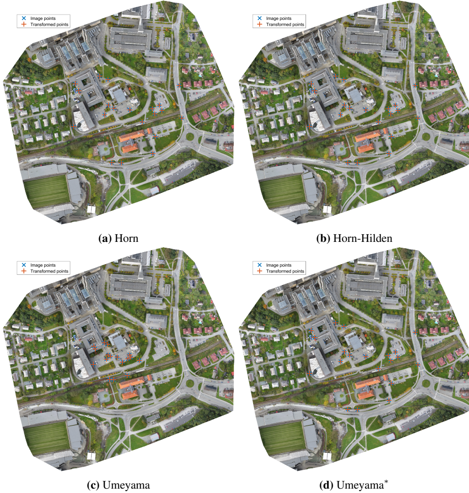
Figure 4.7: Shows the resulting placement of the GCPs in the orthophoto “Lerkendal”. Rematching was turned on for all these. In (a) Horn was used to find the absolute orientation parameters. Horn-Hilden was used in (b), Umeyama in (c), and (d) used Umeyama*. For enlarged versions see Figure B.9, B.12, B.14, and B.16.
