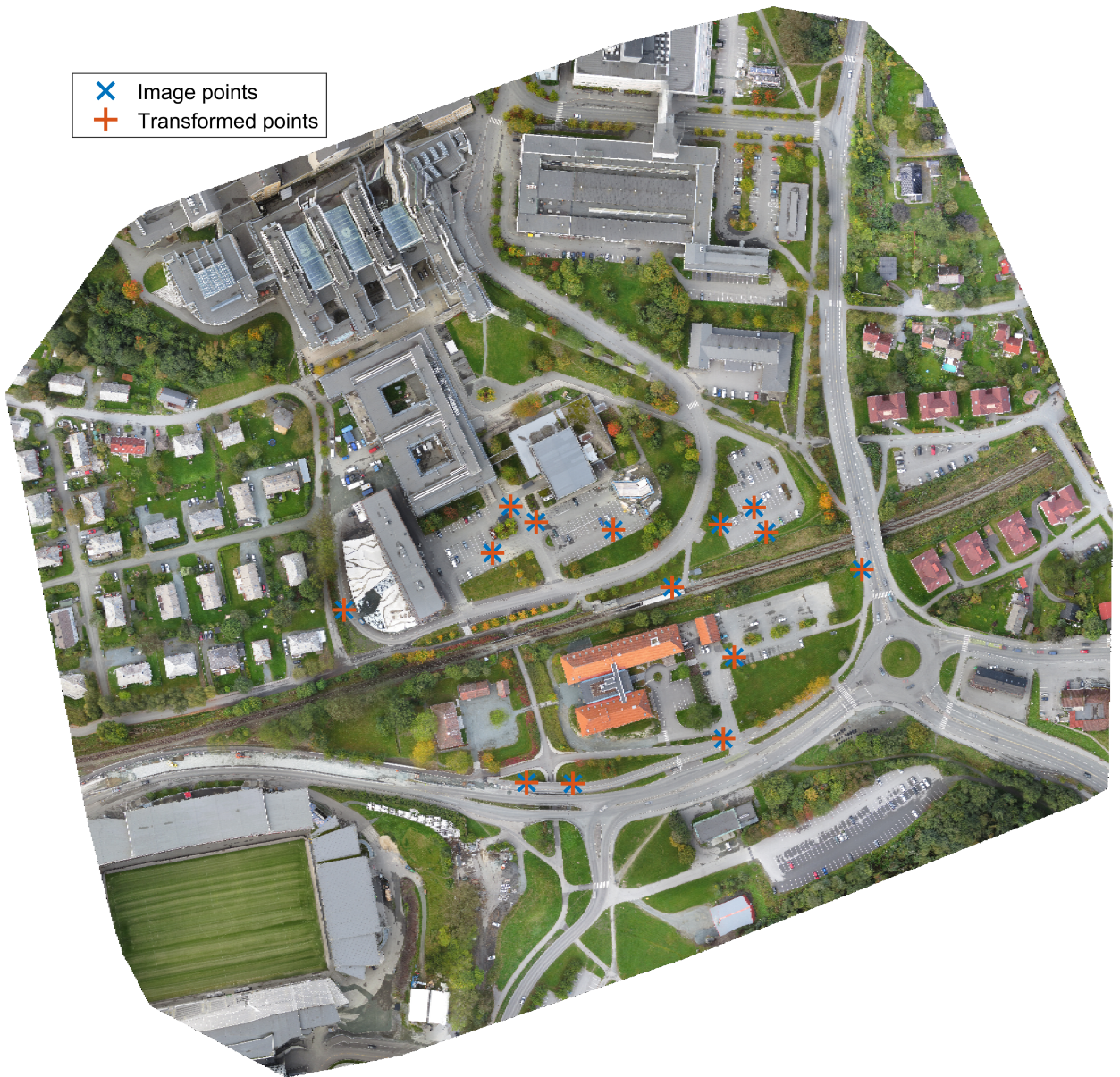
Figure B.11: Lerkendal - Horn-Hilden - without rematching: Shows the orthophoto “Lerkendal”. The blue crosses indicate the areas considered to be a GCP by the prototype when the algorithm proposed by Horn et al. (1988) was used to find the absolute orientation. The orange pluses were calculated from the inverse absolute orientation parameters obtained from Horn-Hilden. The measured-in coordinates of the CM where then inverted to image coordinates and displayed as orange pluses.
