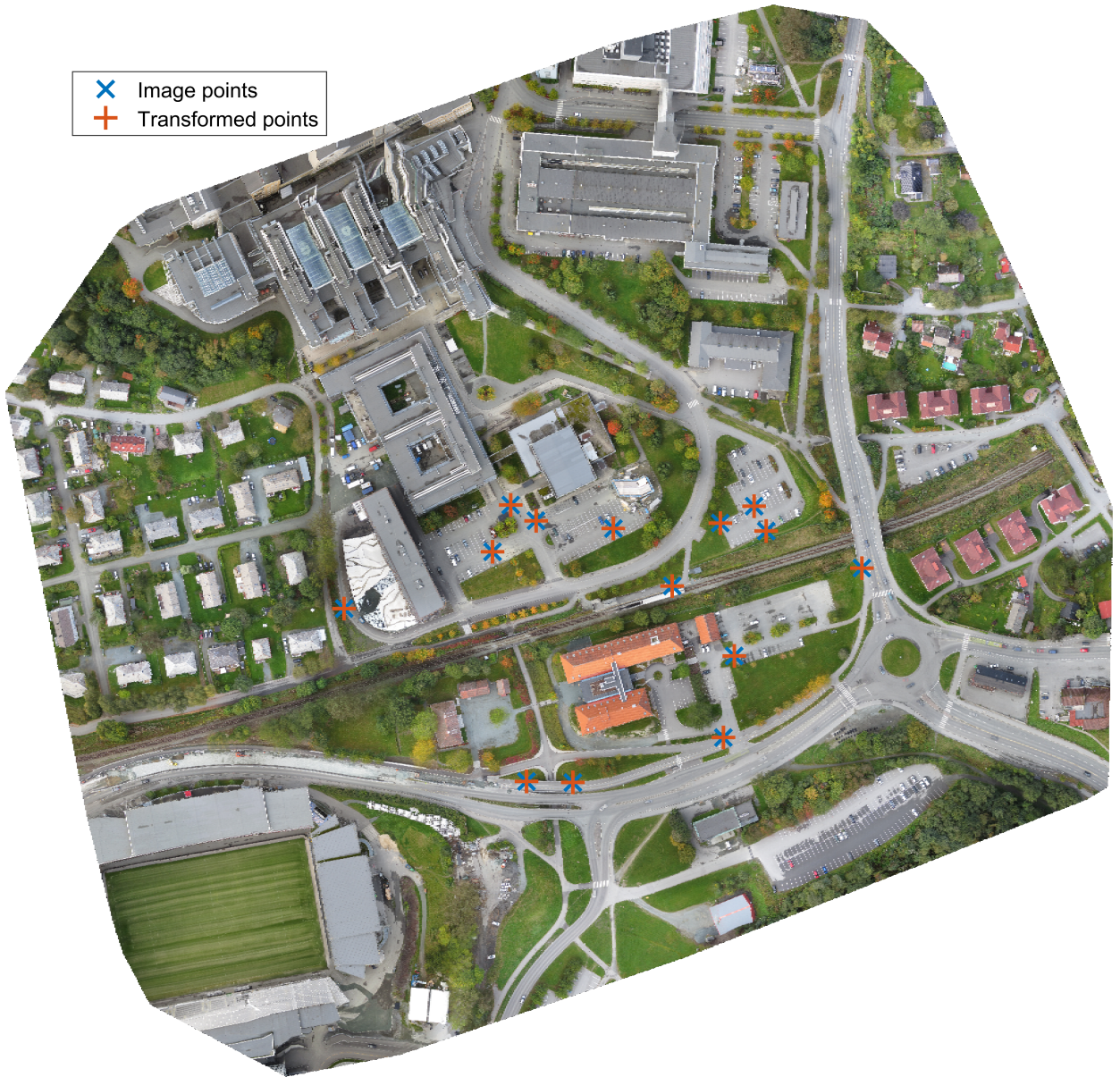
Figure B.15: Lerkendal - Umeyama* - without rematching : Shows the orthophoto “Lerkendal” . The blue crosses indicate the areas considered to be a GCP by the prototype when the algorithm proposed by Umeyama (1991) was used to find the absolute orientation. Instead of using the proposed scale factor, however, the scale factor is calculated as proposed in Horn (1987). The orange pluses were calculated from the inverse absolute orientation parameters obtained from Umeyama*. The measured-in coordinates of the CM were then inverted to image coordinates and displayed as orange pluses.
