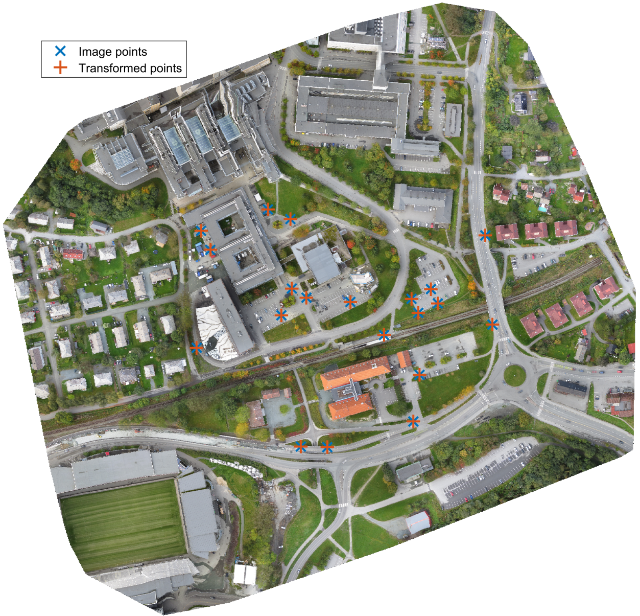
Figure B.9: Lerkendal - Horn - with rematching : Shows the orthophoto “Lerkendal” . The blue crosses indicate the areas considered to be a GCP by the prototype when the algorithm proposed by Horn (1987) was used to find the absolute orientation. The orange pluses were calculated from the inverse absolute orientation parameters obtained from Horn. The measured-in coordinates of the CM where then inverted to image coordinates and displayed as orange pluses.
