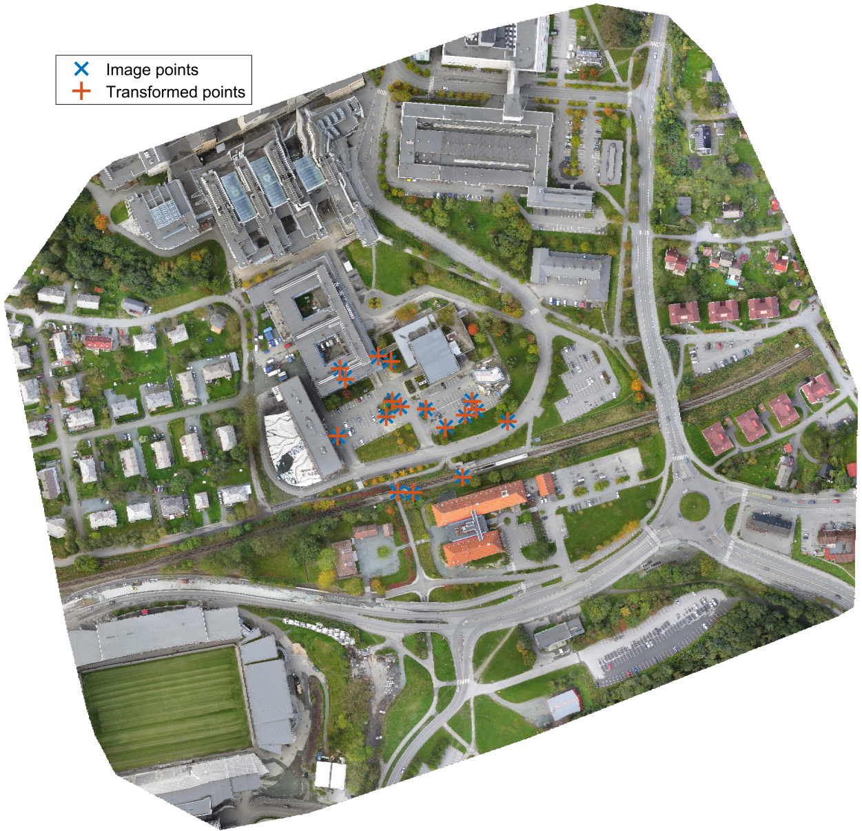
Figure B.14: Lerkendal - Umeyama - with rematching : Shows the orthophoto “Lerkendal” . The blue crosses indicate the areas considered to be a GCP by the prototype when the algorithm proposed by Umeyama (1991) was used to find the absolute orientation. The orange pluses were calculated from the inverse absolute orientation parameters obtained from Umeyama. The measured-in coordinates of the CM where then inverted to image coordinates and displayed as orange pluses.
