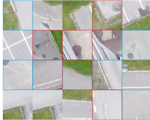
Figure 4.2: An overview over which GCPs were consistently found (blue) and those that were consistently not found (red). The order of the GCPs is the same as in Figure 3.7; i.e. “New1” at the top left corner, and “P18” in the lower right corner with the rest of the points in ascending order. Figure B.17 and B.18 show larger versions of these two images.
