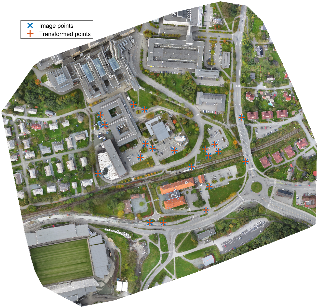
Figure B.12: Lerkendal - Horn-Hilden - with rematching : Shows the orthophoto “Lerkendal”. The blue crosses indicate the areas considered to be a GCP by the prototype when the algorithm proposed by Horn et al. (1988) was used to find the absolute orientation. The orange pluses were calculated from the inverse absolute orientation parameters obtained from Horn-Hilden. The measured-in coordinates of the CM were then inverted to image coordinates and displayed as orange pluses.
