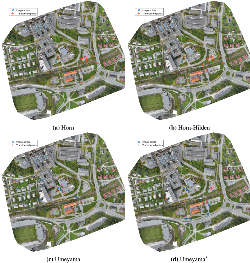
Figure 4.6: Shows the resulting placement of the GCPs in the orthophoto “Lerkendal”. Rematching was turned off for all these. In (a) Horn was used to find the absolute orientation parameters. Horn-Hilden was used in (b), Umeyama in (c), and (d) used Umeyama*. For enlarged versions see Figure B.10, B.11, B.13, and B.15.
