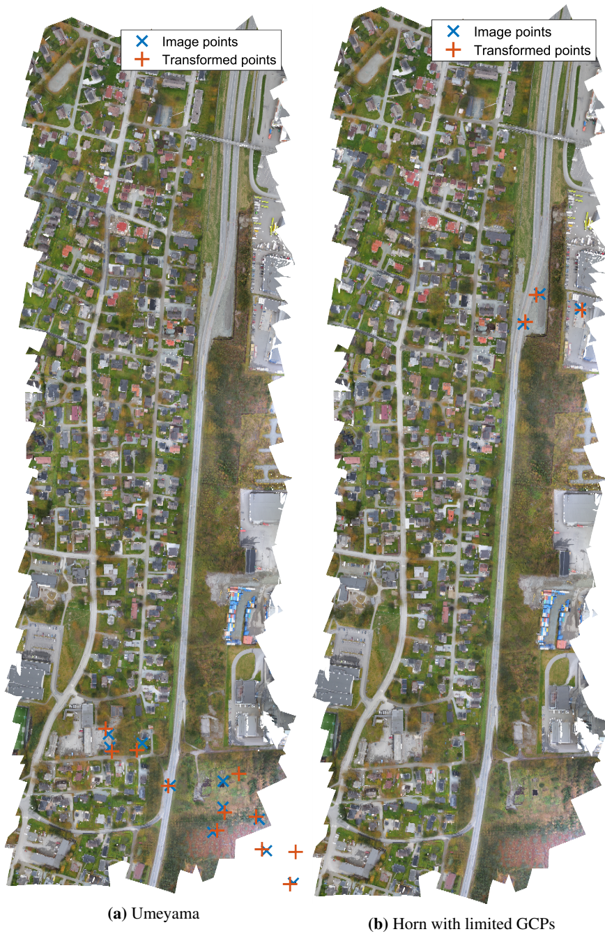
Figure 4.13: Shows the resulting placement of the GCPs in the orthophoto “E6”. Rematching was turned on. (a) shows the results when using Umeyama, while (b) is obtained by using Horn, but the list of GCPs was limited to only the points visible in the orthophoto.
