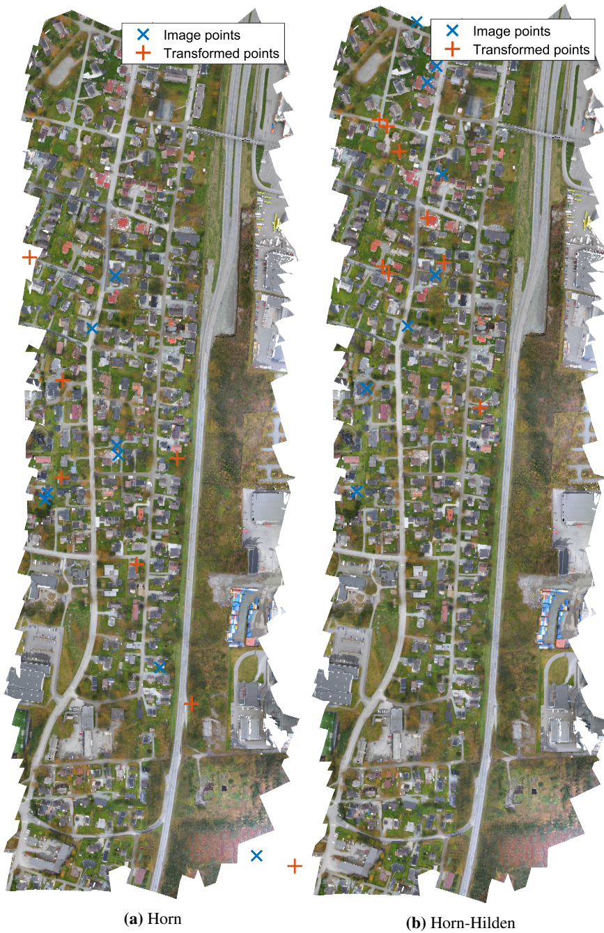
Figure 4.12: Shows the resulting placement of the GCPs in the orthophoto “E6”. Rematching was turned on. (a) shows the results when using Horn, while (b) is obtained by using Horn-Hilden.
