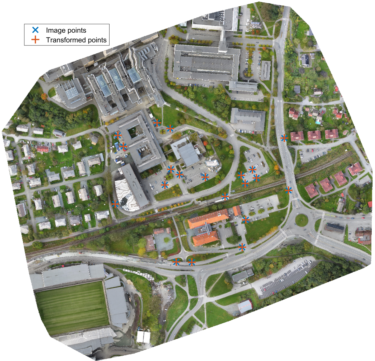
Figure B.16: Lerkendal - Umeyama* - with rematching: Shows the orthophoto “Lerkendal” . The blue crosses indicate the areas considered to be a GCP by the prototype when the algorithm proposed by Umeyama (1991) was used to find the absolute orientation. Instead of using the proposed scale factor, however, the scale factor is calculated as proposed in Horn (1987). The orange pluses were calculated from the inverse absolute orientation parameters obtained from Umeyama*. The measured-in coordinates of the CM where then inverted to image coordinates and displayed as orange pluses.
