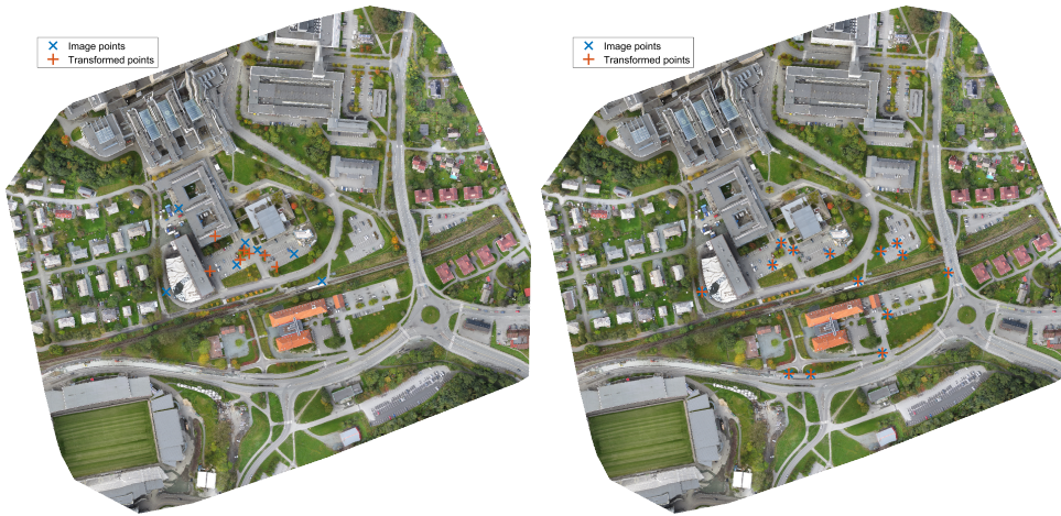
(a) Illustrates the placement of image GCPs, and transformed GCPs when the scale factor proposed by Umeyama (1991) is used. (b) Illustrates the placement of image GCPs, and transformed GCPs when the scale factor proposed by Horn (1987) is used.
