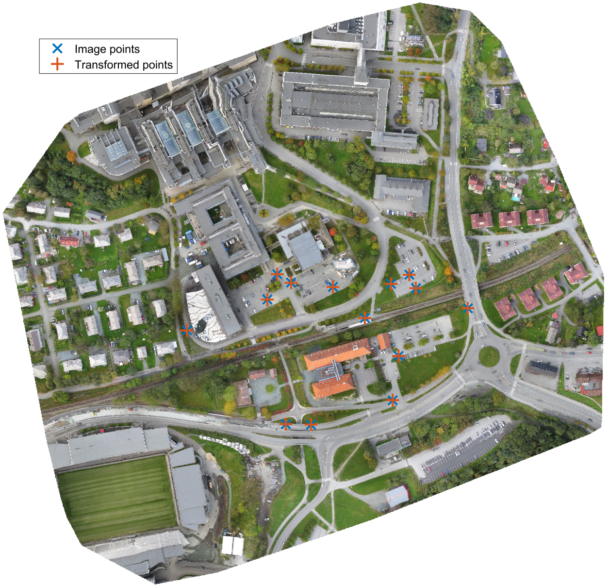
Figure B.10: Lerkendal - Horn - without rematching : Shows the orthophoto “Lerkendal”. The blue crosses indicate the areas considered to be a GCP by the prototype when the algorithm proposed by Horn (1987) was used to find the absolute orientation. The orange pluses were calculated from the inverse absolute orientation parameters obtained from Horn. The measured-in coordinates of the CM where then inverted to image coordinates and displayed as orange pluses.
