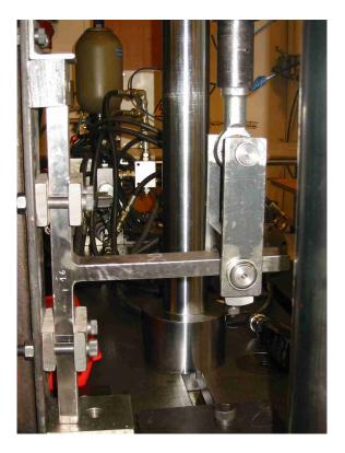
Figure 7.4: T-joint test mounted.
