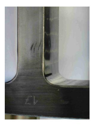
Figure 7.1: T-joint specimen. Standard quarter-circular transition.
