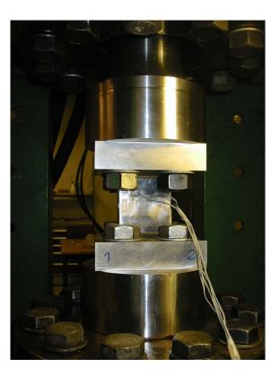
Figure 7.12: Trailing edge transition test mounted.
