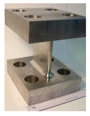
**Figure 7.9:** Circular-shaped trailing edge transition specimen.
