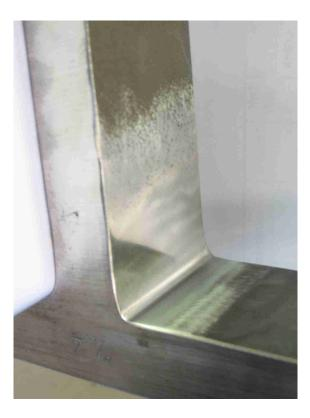
**Figure 7.2:** T-joint specimen. Shape optimised transition (case D).
