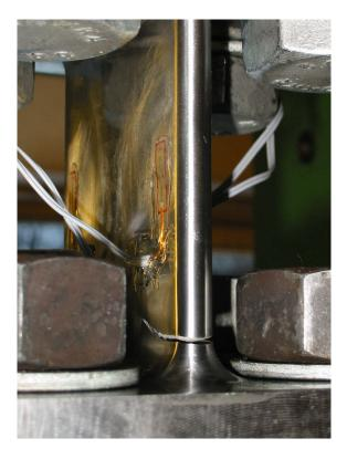
Figure 7.14: Trailing edge test specimen RI. Failure due to crack growing from stress concentration.
