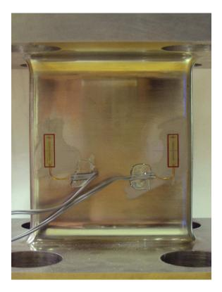
Figure 7.13: Strain gauge placement.
