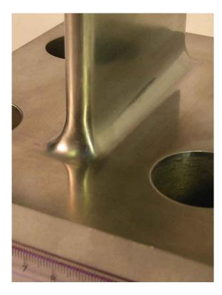
**Figure 7.10:** Shape optimsed trailing edge transition specimen.
