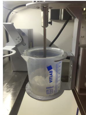
Figure 3.4: Mixing SiR in vacuum chamber
