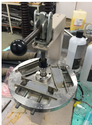
Figure 3.7: SiR specimens aligned to rotating disc
