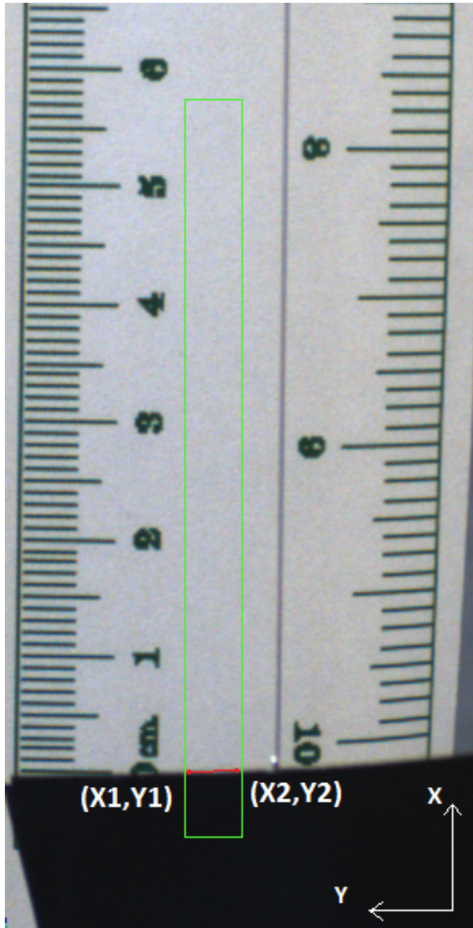
Figure D.1: Camera image with ROI (green square) and detected edge (red line). The axes are added after the image is captured for reference.
