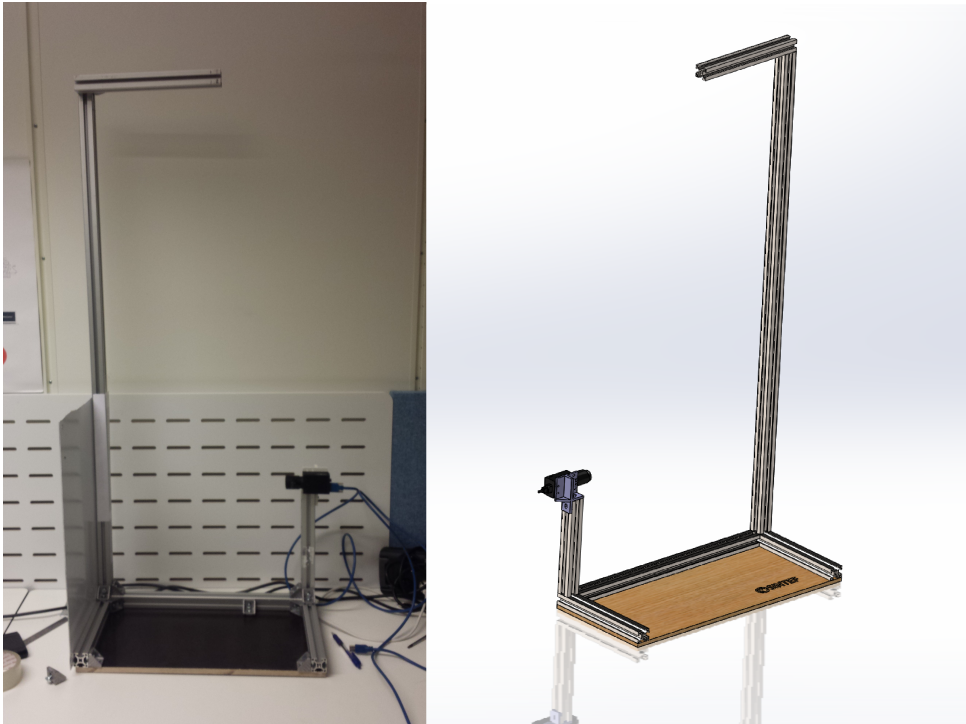
Figure E.2: The actual test rig (to the left) compared to the CAD -sketch (to the right).
