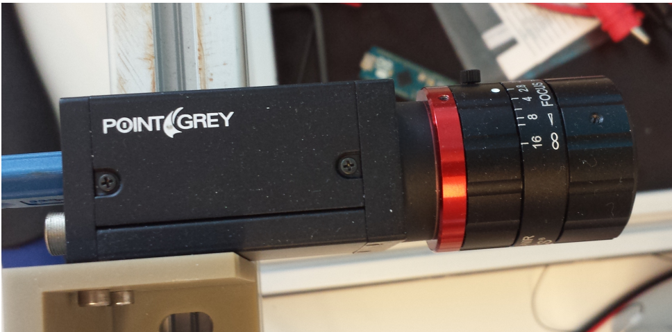
Figure E.1: Image of the camera used to make the measurements of the actual displacement ( D_S ).
