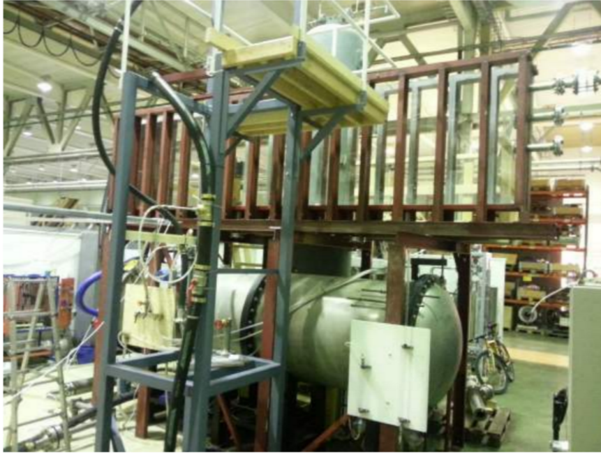
Figure 5.1: Overview of the rectangular test separator on top of the grey feed separator [28]
