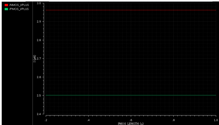
Figure 19: Incorrect NMOS and PMOS leakage currents as a function of PMOS length
