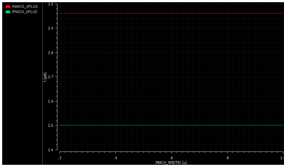
Figure 20: Incorrect NMOS and PMOS leakage currents as a function of PMOS width
