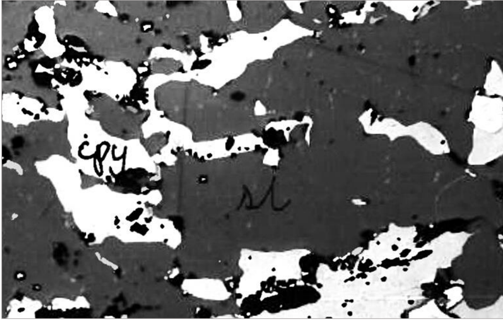
Figure 29: Excerpt of Figure 10, modified with higher contrast. Indications of 'chalcopyrite disease' in sphalerite (sl), see text for further explanation. Figure modified from Bakke (1975).
