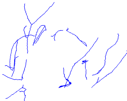
Figure 4.6: Centerline extraction with Circle Fitting, no-denoising dataset 2
