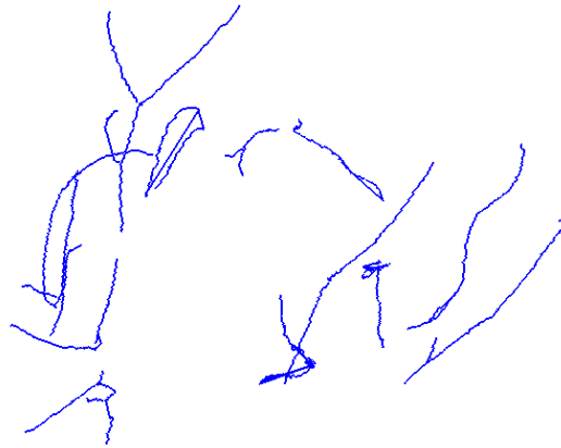
Figure 4.38: Centerline extraction with Circle Fitting, Gaussian Smoothing High Parameters and Non-local Means dataset 2
