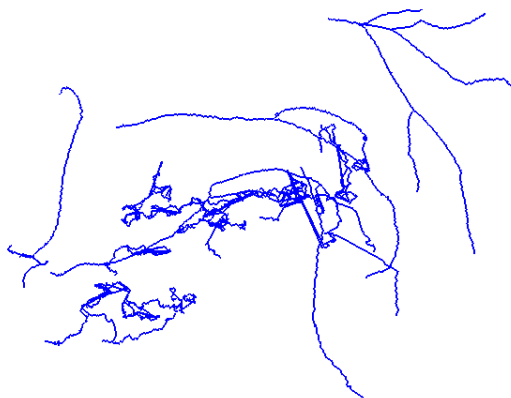
Figure 4.37: Centerline extraction with Circle Fitting, Gaussian Smoothing High Parameters and Non-local Means dataset 1
