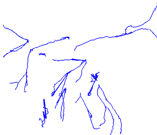
Figure 4.14: Centerline extraction with Circle Fitting, Gaussian Smoothing Low Parameters dataset 2
