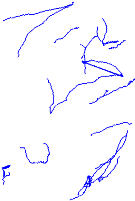
Figure 4.13: Centerline extraction with Circle Fitting, Gaussian Smoothing Low Parameters dataset 1
