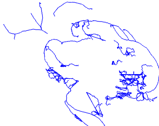
Figure 4.33: Centerline extraction with Vesselness Filter, Gaussian Smoothing High Parameters and Non-local Means dataset 1
