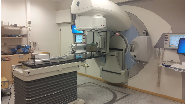
Figure 2.11: Conventional linac at St. Olavs Hospital, shown with the Delta4 phantom placed on the patient treatment table.
