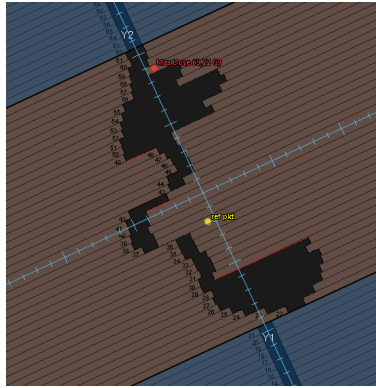
Figure 2.6: The field opening of the MLC leaves seen from BEV in RayStation TPS. Three MLC flanks are indicated with a red marker.
