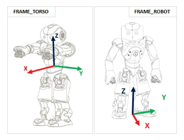
Figure 2.5: **Choosing the frame:** This is Nao's *torso* and *robot* frame. The torso fram is what we will be using in this project. Picture from (Cartesian Control 2-1, 2015).
