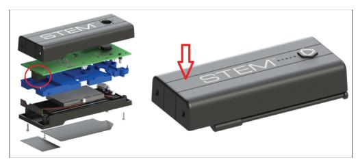
Figure 1.3: **STEM-pack:** The pack's electromagnetic tracker is placed as shown in red. Image from (08/01/2014 - STEM Pack Details, 2014).
