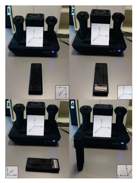
Figure 3.17: **Changing frame for the tracker:** Here are the four steps for changing the frame of the tracker to match the frame of the robot. The rotating frame of the tracker is shown in the bottom left corner of each step, while the frame of the base station remains fixed.
