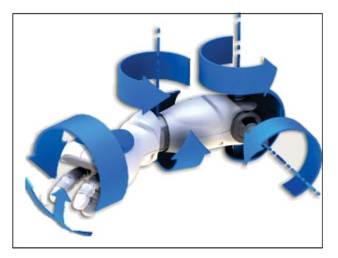
Figure 3.16: **Actual DOFs:** This figure shows the arm effectors 5 DOFs, and about which axis each of the joints rotates. As shown here, the elbow yaw is a rotation about the overarm, whereas the wrist yaw is a rotation about the underarm. Picture taken from Choreographe.
