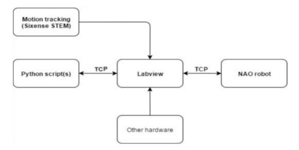
Figure 2.2: **Old program:** In the original program, LabVIEW was used as a centre of communication. This meant that it was necessary to have TCP-connections both between the Python-script and LabVIEW, and between LabVIEW and the NAO robot.
