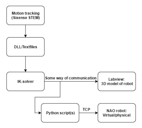
Figure 2.4: **New system structure:** In this new system, data from the STEM-system would be collected using DLL-files or text-files. The data would then be sent to the IK-solver, which would hopefully return the angles necessary to realize the movement. These angles would then either be sent to LabVIEW for testing, or to a Python-script to control the actual robot.
