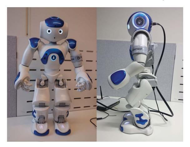
Figure 2.7: **StandInit:** This is the pre-set position *StandInit*, which is a good start position for controlling NAO's arms.
