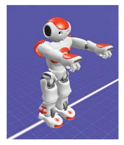
Figure 2.11: **Virtual NAO:** This is the virtual robot in Choreographe. All methods from the NAOqi SDK (see section 2.2) could be tested on this model, and it would behave almost exactly like the real robot.
