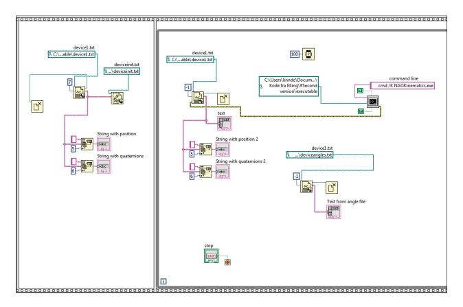
Figure 3.13: **Continuous IK-solver testing:** The exe-file is calculating the movement between the tracker data in deviceinit.txt with the data currently written in device1.txt. The data in the last file is continuously updated by Øye's program, see section 3.2.2.
