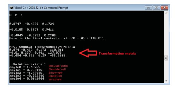
Figure 3.8: **Valid solution:** When manually setting the transformation matrix in the C++-script to match the transformation matrix for NAO's left hand when being in the *Initial Position*, the IK-solver returned the output shown above for the five angles in NAO's left arm effector.
