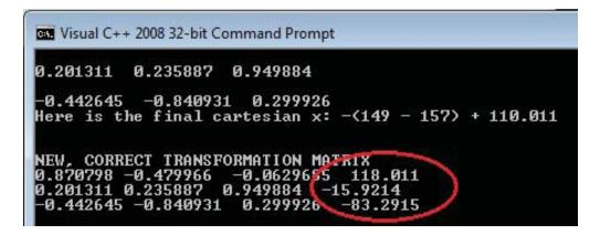
Figure 3.11: **Wrong output:** It is clear that the calculated Cartesian coordinates do not match what is known to be the correct answer. Somewhere in the program there must be some mathematical error.
