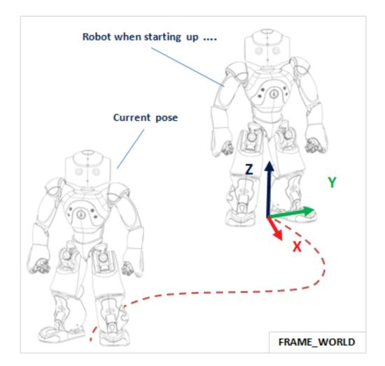
Figure 2.6: **Choosing the frame:** This is Nao's *world* and *robot* frame. Theoretically, this should be able to track NAO's complete movement from startup. Picture taken from (Cartesian Control 2-1, 2015).
