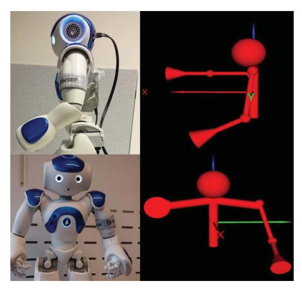
Figure 3.9: **Matching angles:** When setting the five angles on the left arm of the simple 3D-model on the right, the final position and orientation of the arm matched the actual robot in its *Initial position*. As mentioned in section 3.5, testing was only done on the left arm of the robot.
