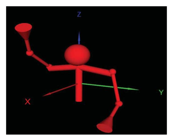
Figure 2.10: **Robot model:** This is the 3D-model created in LabVIEW to perform tests of the system. The model is similar to NAO's torso, and the arms have the same DOFs, so that the different joints moves just like NAO's joints.
