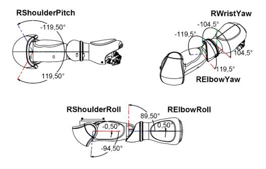
Figure 2.8: **Arm joints:** Here we can see how the five DOFs in NAO's right arm is distributed. Picture from (NAO Technical Guide: H25 - Joints - V3.2, 2012).
