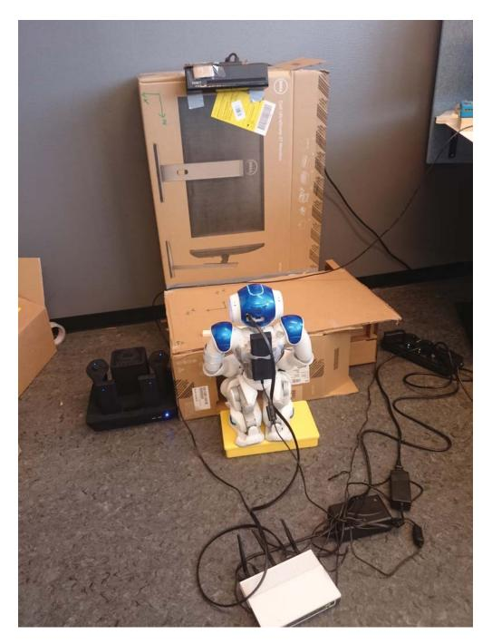
Figure 3.20: **Summer lab:** Here is the complete system from the summer project. The rig is made of cardboard because of Sixense STEM's metal sensitivity, and the robot is connected to the Internet through a cable because of the WiFi-sensitivity.
