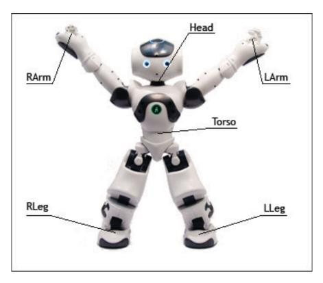
Figure 2.9: **Control points:** The sensors that make up the control point for NAO's effectors. As shown, the sensor in NAO's arm is located in the centre of the hand (Cartesian Control, 2012).
