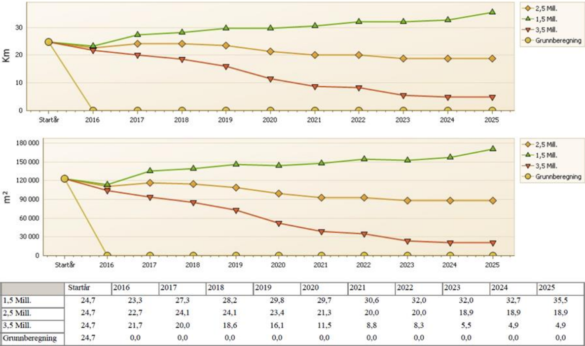
Figure 2:3- Overview of how the length and area of low standard roads will evolve over 10 years with various maintenance budget. (Finnerud and Sweco, no date)
