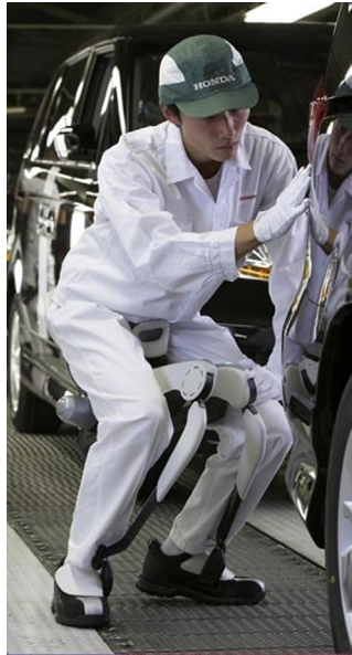
Honda Bodyweight Support Assist Device
