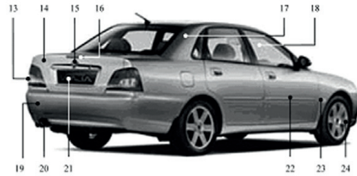
Figure 2B. Selected Car Components on 3 quarter rear view. Note: (13) Tail lamp; (14) Trunk lid; (15) Rear emblem; (16) 3rd brake light; (17) C-pillar; (18) B-pillar; (19) Rear bumper; (20) Exhaust; (21) Rear plate number; (22) Body trim; (23) Side signal; and (24) Wheel.
