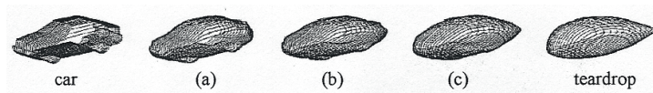
Figure 2. Weighted averaging shapes from a car and the teardrop shape under ratios of (a) 70/30, (b) 50/50, and (c) 30/70 (Source: Chen and Parent [11])
