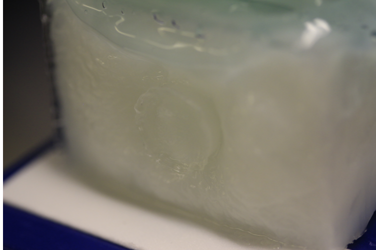
Figure 3.6: Closeup of the phantom, showing the cyst
