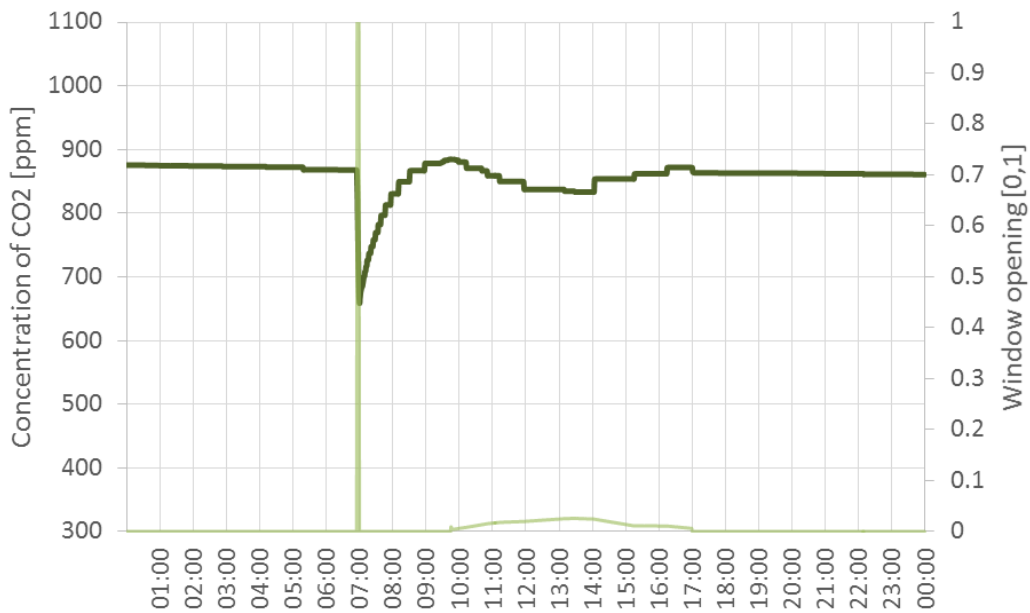
Figure 52 Concentration of CO 2 and opening frequency on cold day, Hybvent 40_60
