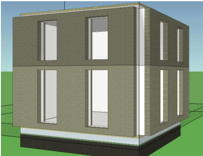
Figure 37 Windows mounted flush interior IDA
