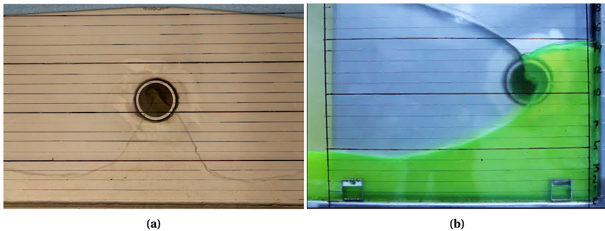
Figure 4.13: Steady state pictures of the water jump for high flow rates and small annulus gaps. Here (a) shows the situation for symmetric inflow, while (b) [17, page 41] shows one-sided inflow.
