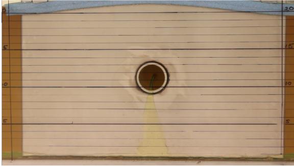
Figure 3.15: Test with roof at \delta = 5 [mm], WL = 10 [mm] and valve position 4.
