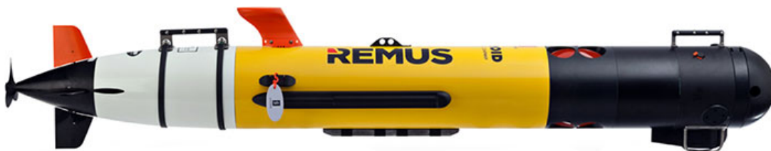
Figure 1.1: Hydroid REMUS 100 AUV (Kongsberg Maritime, 2015).
