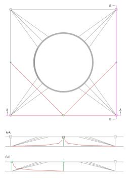
Figure 8.15: Concept of external mooring system
