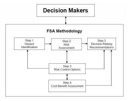
Figure 3.1: Flow chart of FSA methodology (IMO, 2013)
