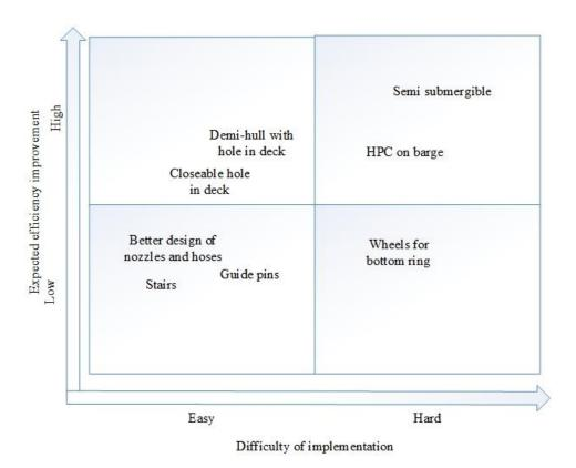
Figure 7.8: Prioritising matrix, Design of cleaning barge
