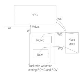
Figure 8.34: Concept of storing tank for ROV/RONC
