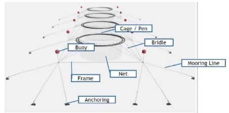
Figure 4.4: Typically mooring system for fish farm (Søreide, 2016)
