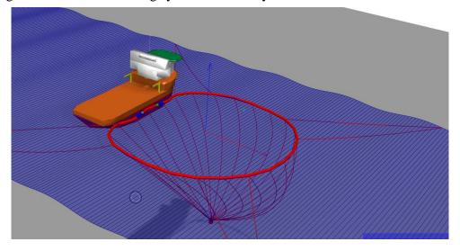
Figure 4.8: Impact on floating collar from vessel moored to the windward side of the cage
