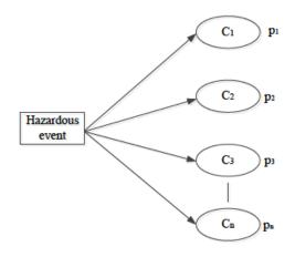
Figure 3.8: Consequence spectrum (Rausand, 2011)
