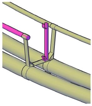
Figure 8.13: Concept with hook for fixed mooring line
