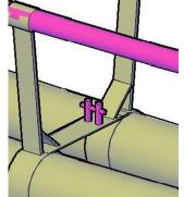
Figure 8.14: Concept mooring fastening specific for vessel
