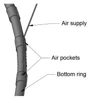
Figure 8.28: Concept of external buoyancy system for bottom ring
