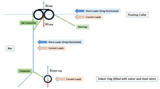
Figure 4.6: Environmental forces on a net cage (Søreide, 2016)
