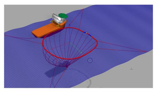
Figure 4.9: Impact on floating collar from vessel moored with the environment towards the bow
