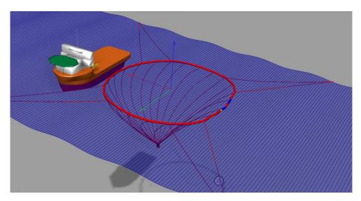
Figure 4.10: Impact on floating collar from vessel moored to the leeward side of cage
