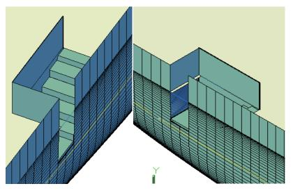
Figure 8.7: Concept design of stairs
