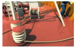
Figure 8.20: Winch bollards delivered by TTS Marine AS (TTSMarine, 2016)
