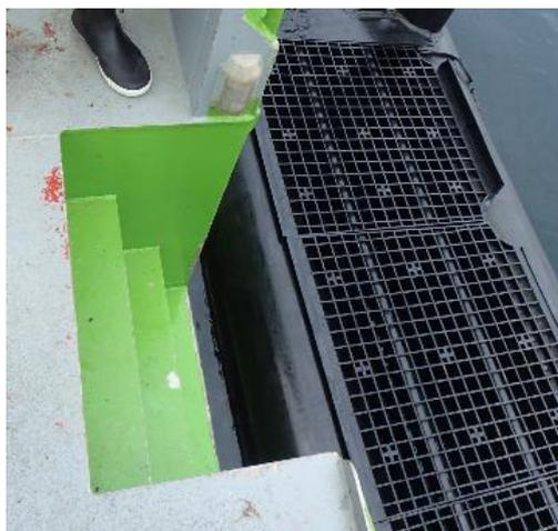
**Figure 8.6: Example of hazardous stair**
