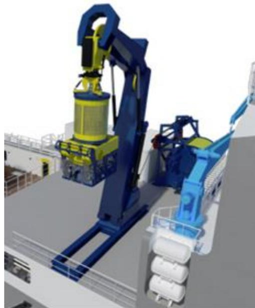
**Figure 8.26: Crane based LARS delivered by Palfinger (Palfinger, 2016a)**
