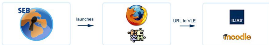
Figure 2.2: Illustration of SEB's architecture. [2].
