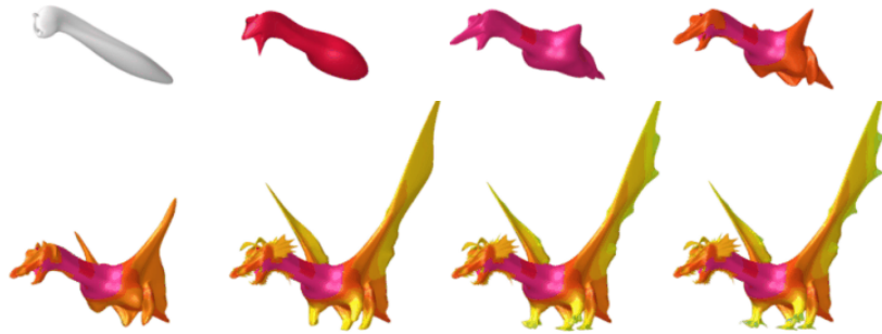
Figure 3.1: The hierarchical levels in Forsey's dragon example (source: www.cs.ubc.ca/nest/imager/ ). The head and the body are modelled with one hierarchical B-spline surface each and pasted together.
