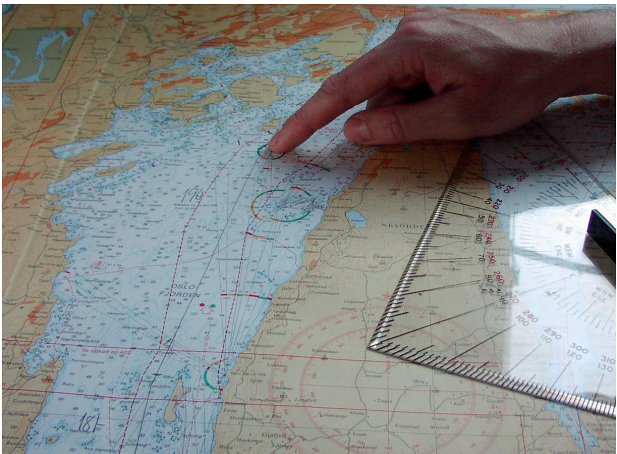
Figure 3-3: The navigation plan shown in a chart. The figures “190” and “181” refer to the compass course to steer.
