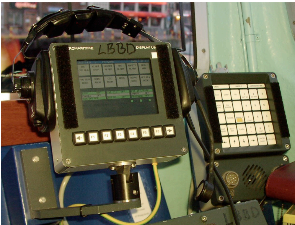
Figure 5-2: The communication system at the commanding officer's position. The system includes the two boxes and the headset.
