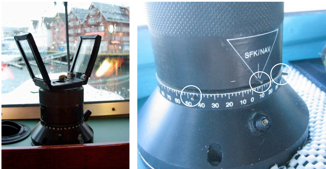
Figure 6-2: The optical bearing device. The three alignment pins and the scale can be seen on the close-up picture to the left.
