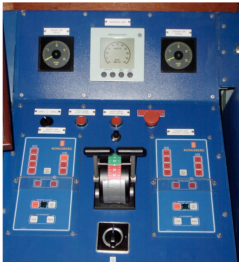
Figure 5-3: The automation interface. The throttles are in the centre, buttons for changing mode are located beside the throttles. Dials representing the engines' rotational speeds are on the upper part of the figure.
