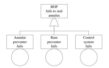
Figure 24: FT for BOP fails to seal annulus.
