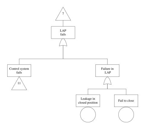
Figure 32: FT "Lower annular fails".
