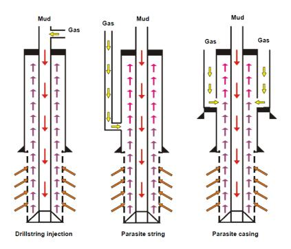
Figure 19: Methods for introducing and circulating fluid in UBD (from Rigpass, 2012).
