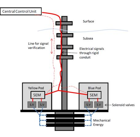
Figure 21: Basic principles of electro hydraulic/MUX control system (from Padøy, 2011).
