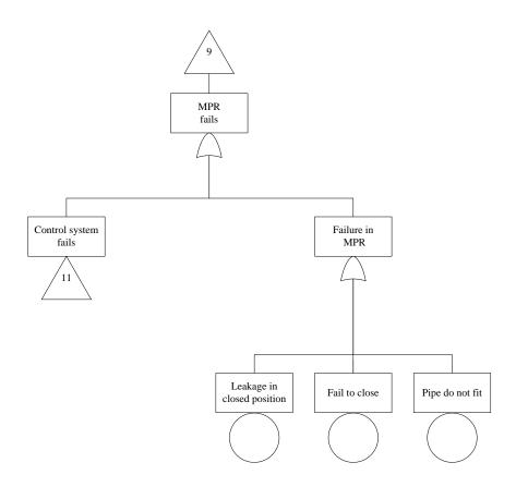
Figure 34: FT "Middle pipe ram fails".
