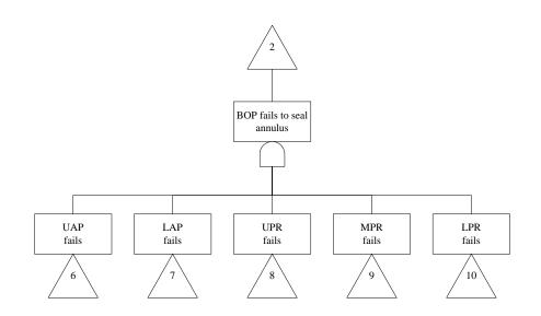
Figure 26: FT "BOP fails to seal annulus"
