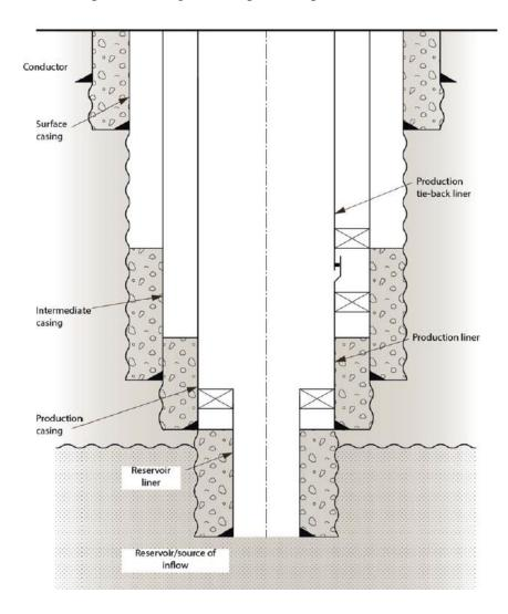
Figure 17: Casing illustration (from NORSOK D-010, 2013).
