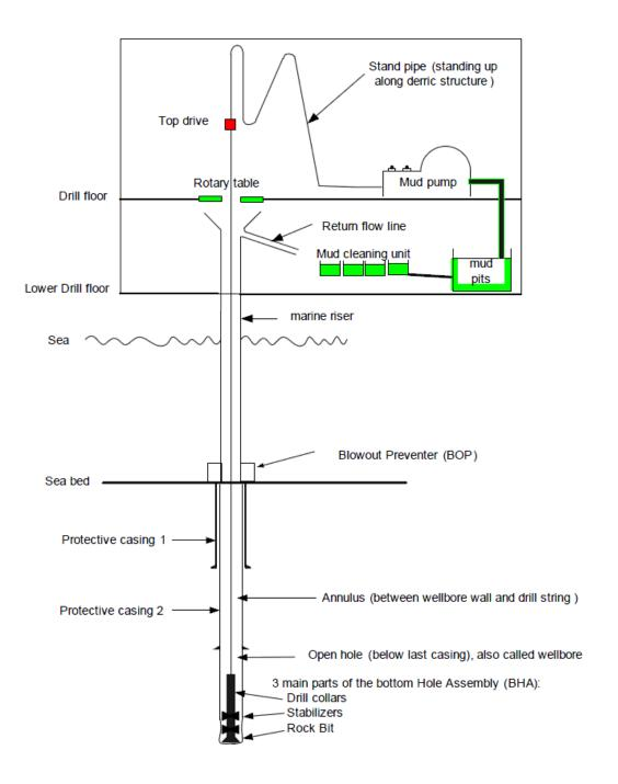
Figure 11: The drilling process (from Skalle, 2011).
