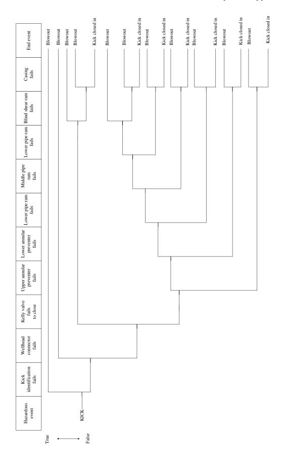
Figure 22: Event tree of barrier elements involved from a kick to blowout during drilling.
