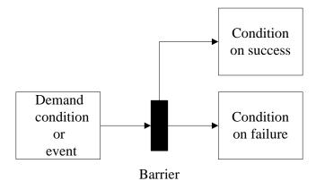
Figure 5: Graphical presentation of a safety barrier in safety-barrier diagrams with two output conditions (from Duijm and Markert, 2009).
