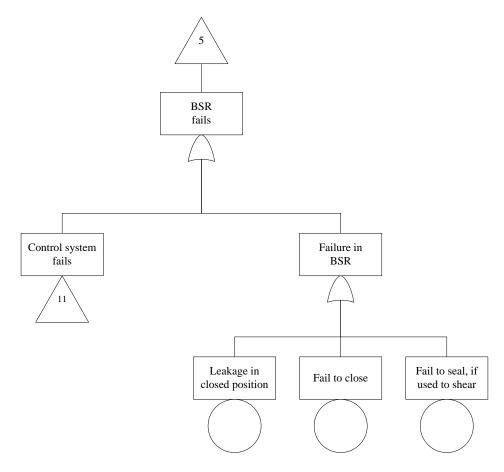
Figure 30: FT "Blind shear ram fails".
