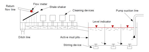
Figure 39: Surface metering of flow out compared to input flow, and of volume change in the pit (from Skalle, 2011).
