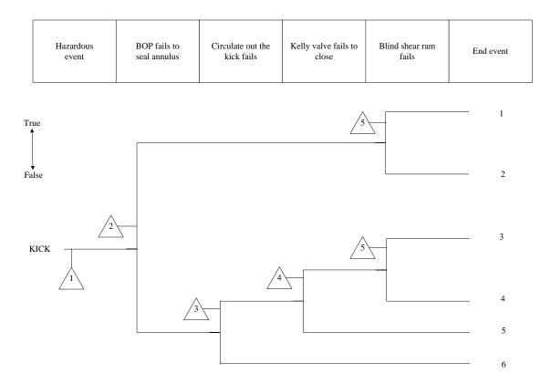
Figure 23: Simplified event tree. Drilling
