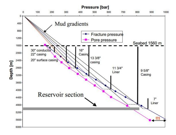
Figure 13: Typical casing program using a 18 <sup>3</sup>/<sub>4</sub>" wellhead system (from TPG 4200, 2012).
