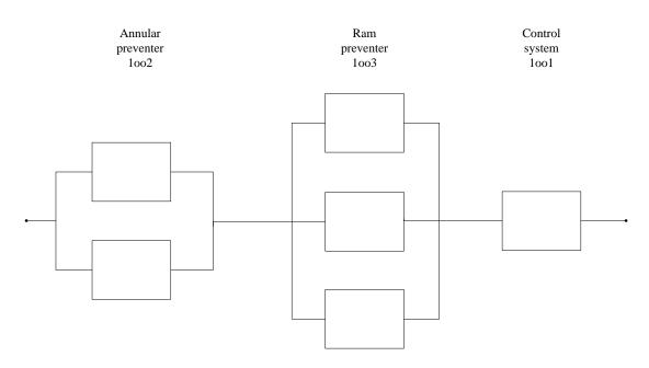
Figure 25: Block diagram of "BOP fails to seal annulus".
