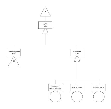
Figure 37: FT "Lower pipe ram fails".
