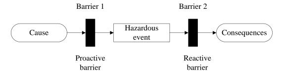
Figure 4: Example of safety barrier diagram (from Rausand, 2011)
