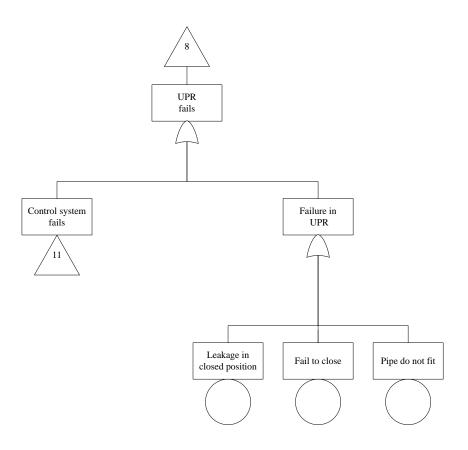
Figure 33: FT "Upper pipe ram fails".
