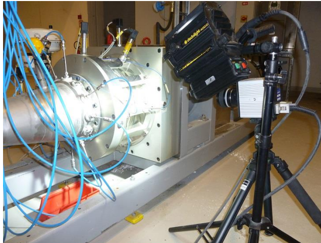
Fig. 20 - Visualization setup: high-speed camera and light focused on the visualization window
