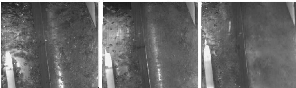
Fig. 33 – Bubble size evolution in the impeller channel; q^* = 100\% , GVF 5 %; from left to right: n = 900, 1200, 1800 rpm
