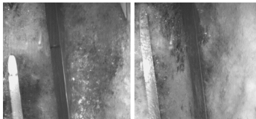
Fig. 42 - Gas pocket interaction and resulting channel blockage and backflow, n = 1200 \text{ rpm} , q^* = 70 \%
