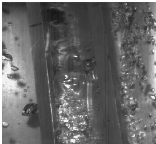
Fig. 5 - Main flow structures and bubbles evolution in the hydraulic channel, from flow visualization on the analyzed pump
