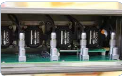
The in-arm electronics module features diagnostic lights that indicate system health.
