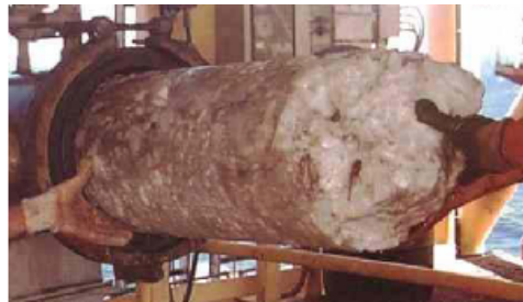
Figure 2.2: A hydrate plug getting removed from a pipeline [3]
