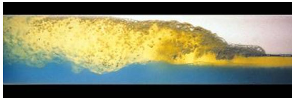
Figure 2.1: Multiphase flow containing two liquid phases and one gas phase.
