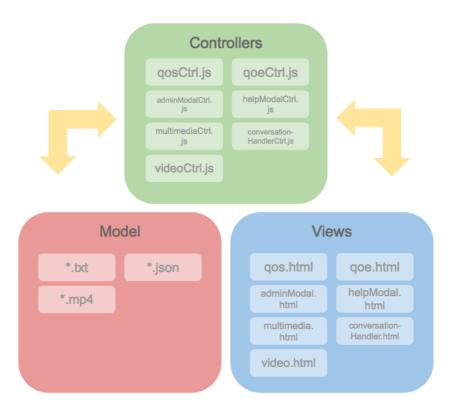
Figure 4.2: Illustration of the system architecture of the WebRTC-dashboard.
