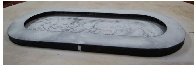
Figure 38: West, open land, initial powder distribution. Note the powder was spread using fingers, hence the pattern
