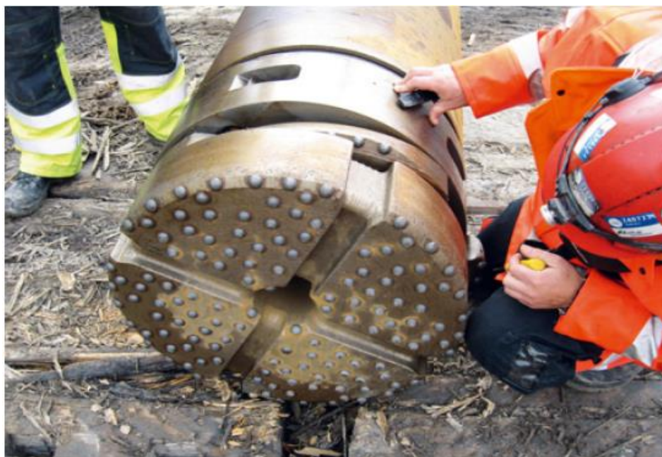
Figur 4-6: Eksempel pilotkrone for RC-boring (Holtmoen 2013)
