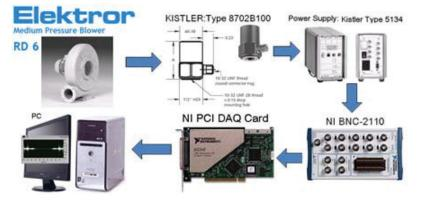
Fig. 6.7 Hardware of Experimental Setup
