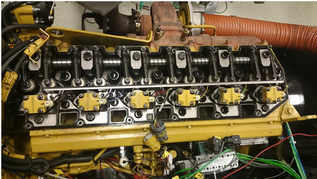
Figure 3.5: Location of injectors with electrical cabling.
